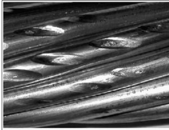
Figure 5.19 ACSR plastic fretting marks on inner layer (Azevedo et al., 2009)
