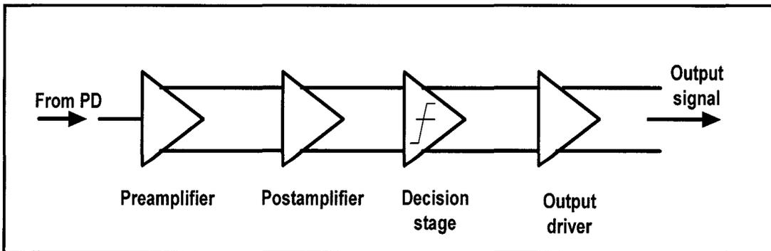
Figure 3-1: A block diagram showing the architecture of an optical receiver circuitry.
