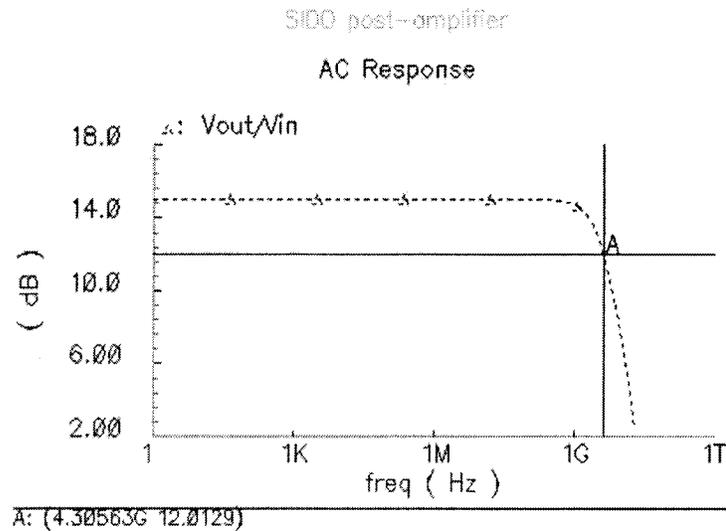
Figure 3-10: Frequency response of the SIDO amplifier.
