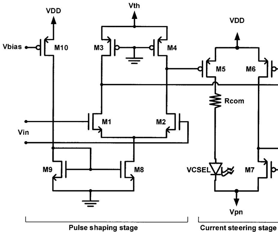
Figure 2-14: Schematic of a fast-discharge laser driver.
