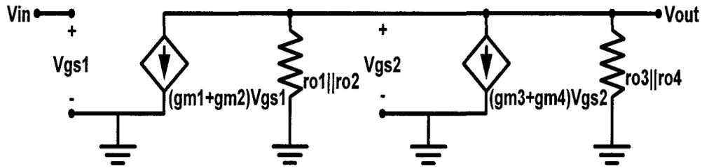
Figure 3-13: Small signal model of the first and second inverter stage in Figure 3-12.
