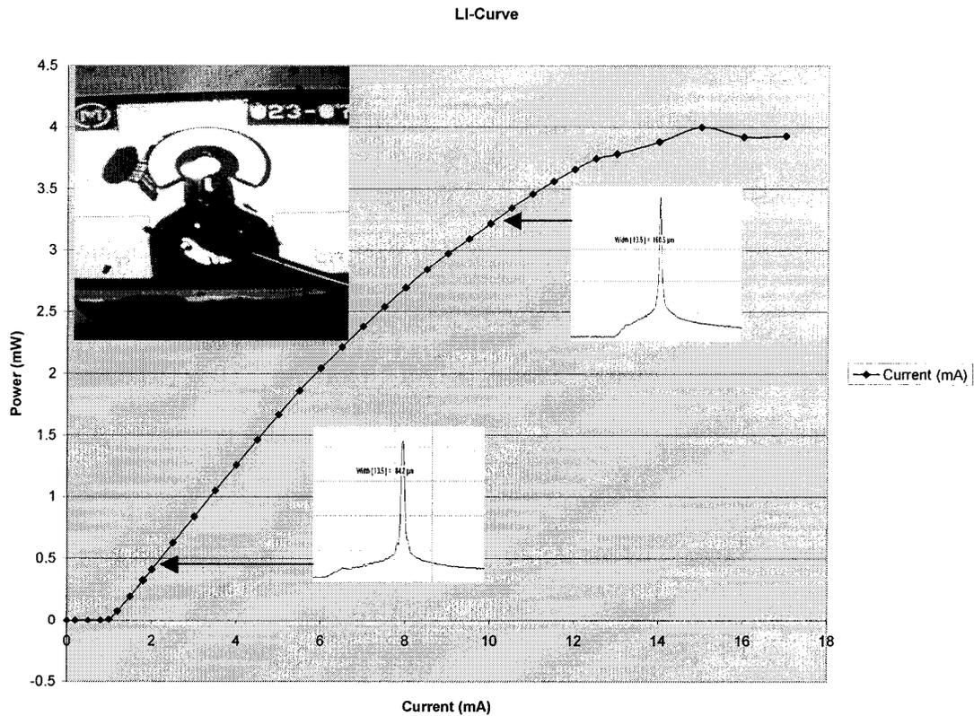
Figure 4-14: Plot of output optical power versus bias current of the VCSEL. Photograph at the top left corner shows the VCSEL biased at threshold. Beam profiles of the output when biased at 2mA and 10mA are also shown.
