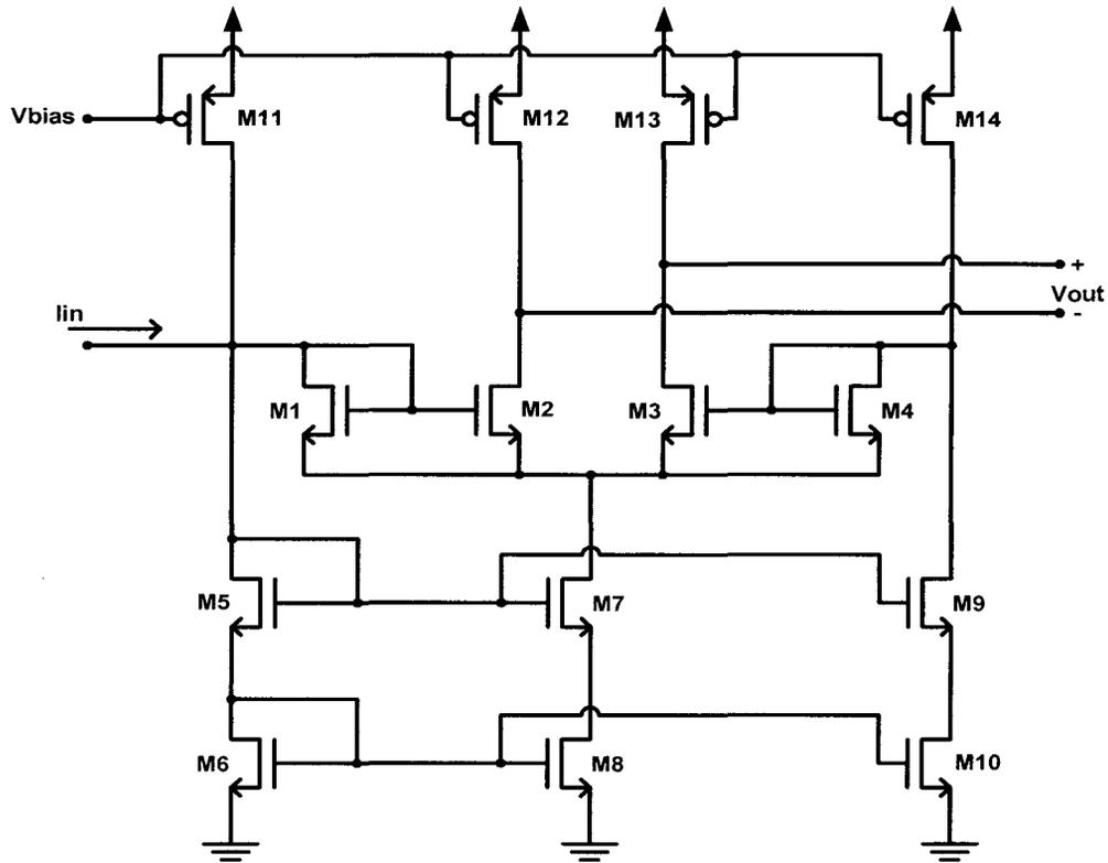
Figure 3-5: Schematic of a current mirror preamplifier.
