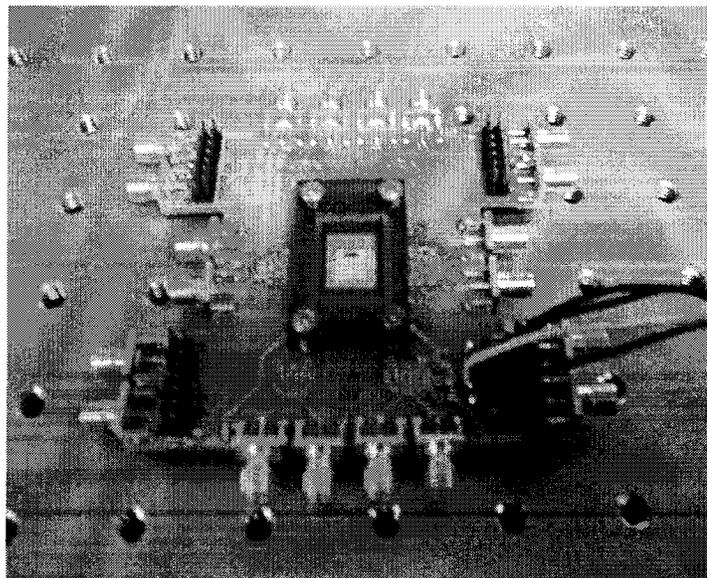
Figure 4-6: Photograph of the CFP80TF printed circuit board test fixture with a chip carrier containing the CMOS receiver and p-i-n photodiode chips.
