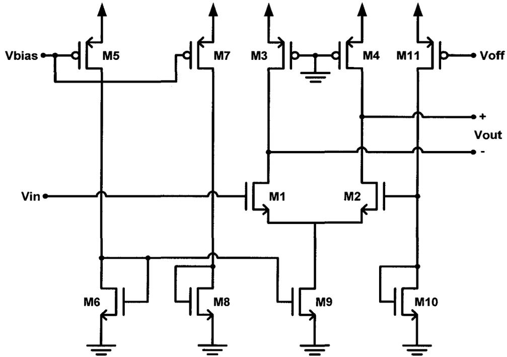
Figure 3-9: Schematic of a single input differential output (SIDO) amplifier.
