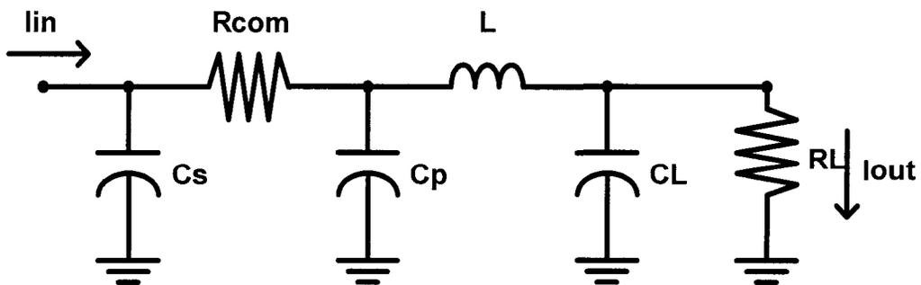
Figure 2-10:  $RLC$  circuit model to simulate the effect of bond-wire parasitic and compensation resistor.
