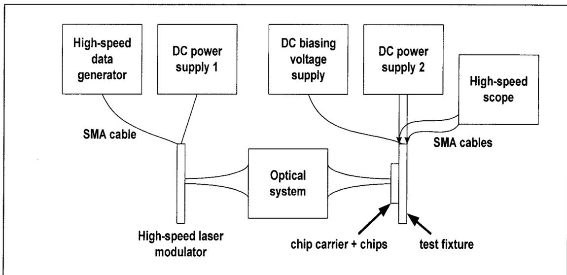
Figure 4-12: Block diagram of the test setup for the optical receiver.
