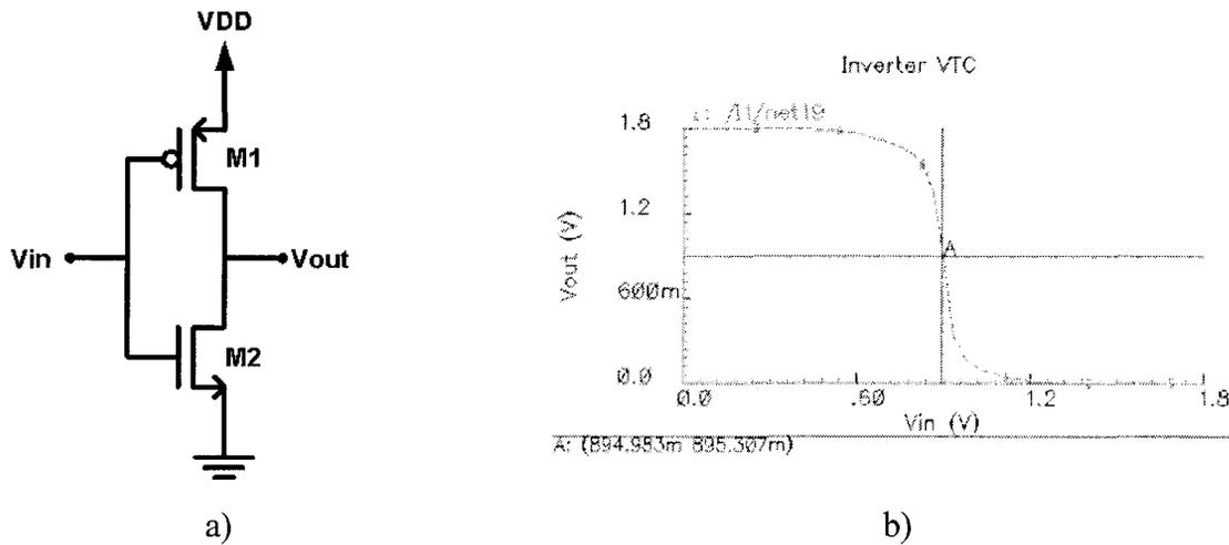
Figure 2-6: a) Schematic of a static CMOS inverter. b) Voltage transfer characteristic (VTC) of a static CMOS inverter.
