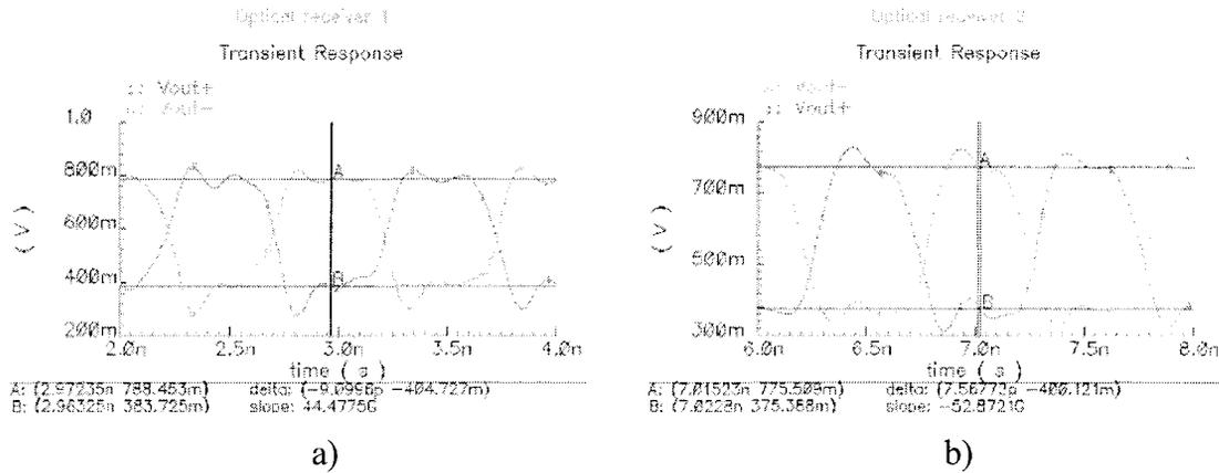
Figure 3-18: Output waveform of the optical receivers designed with a) common gate preamplifier, b) current mirror preamplifier, at 2Gbps.
