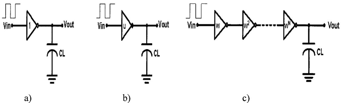
Figure 2-7: a) A minimum-size buffer, b) a buffer  $u$  times the minimum size, c) cascade of  $N$  buffers with increasing gate size, connected to load capacitance,  $C_L$ .
