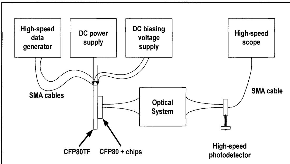
Figure 4-8: Block diagram of the test setup for the optical transmitter.
