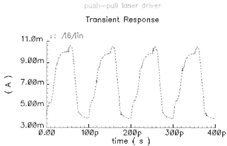
Figure 5-1: Output current of the push-pull laser driver without the parasitic of bond wires, modulating at 20Gbps.
