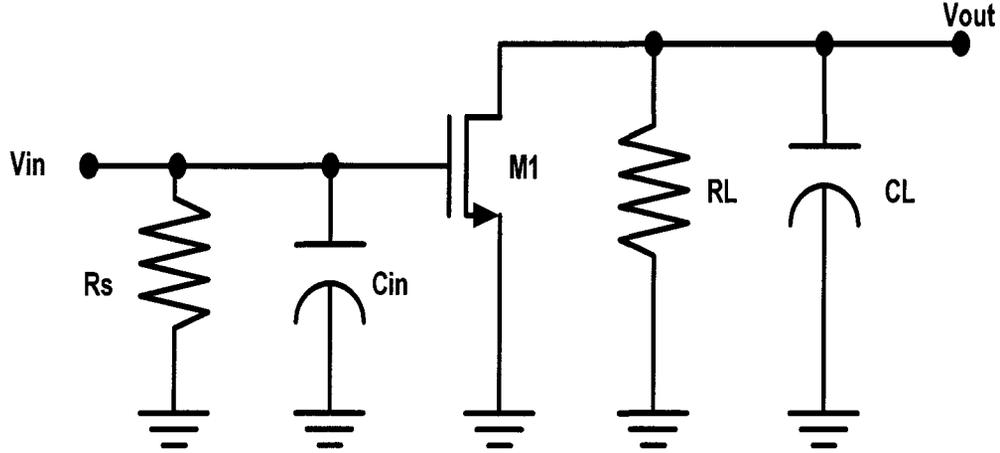
Figure 2-3: Half-circuit equivalent of the GCFD amplifier for frequency analysis.
