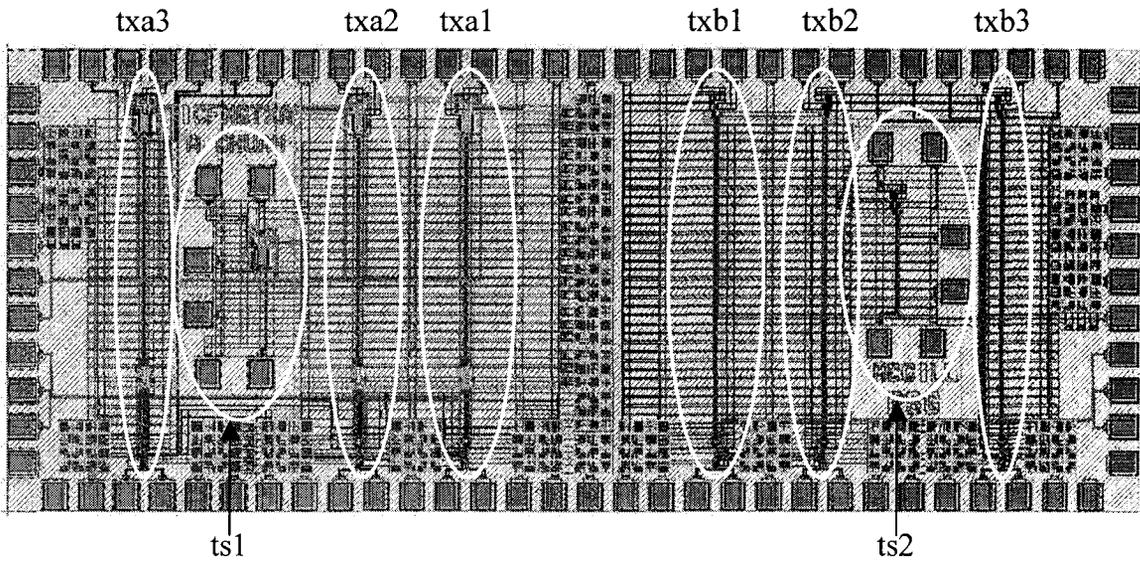
Figure 4-1: Layout of the optical transmitter chip.
