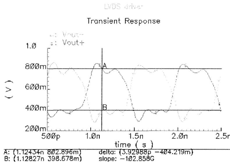
Figure 3-16: Output waveforms of the LVDS driver, simulated at 2Gbps. The markers measure the output voltage swing at 400mV.
