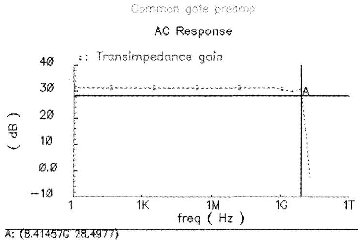
Figure 3-4: Frequency response of the common gate preamplifier (shown in Figure 3-3).
