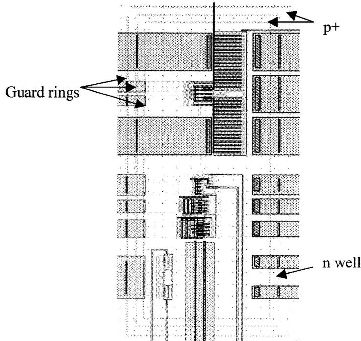
Figure 4-3: Layout of analog circuits (preamplifier and post-amplifier) with their guard rings.
