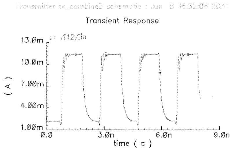
Figure 2-13: Transient response of the current provided to VCSEL by the current steering laser driver, at 1Gbps.
