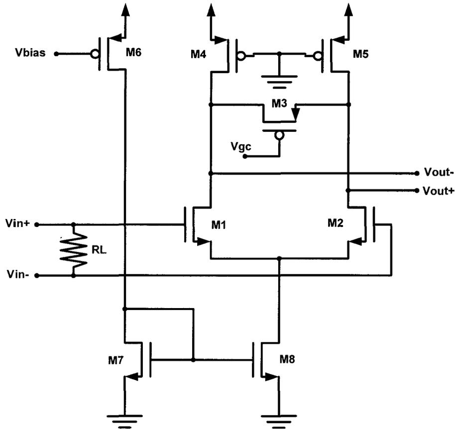
Figure 2-2: Schematic of the gain-controlled fully differential (GCFD) amplifier.
