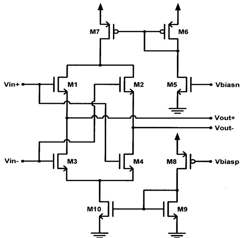
Figure 3-15: Schematic of a LVDS driver implemented in the optical receivers.
