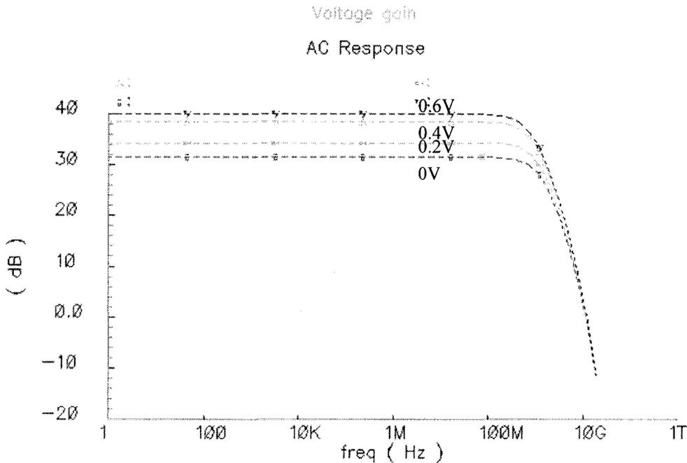
Figure 3-8: Frequency response of the post-amplifier for  $V_{gc}= 0V, 0.2V, 0.4V,$  and  $0.6V$ .
