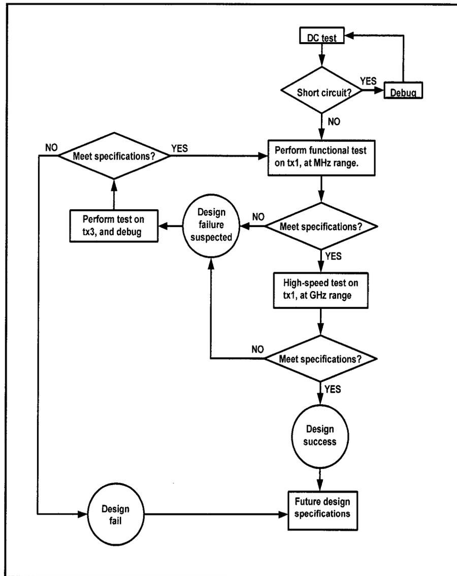
Figure 4-10: A flowchart summarizing the test process for an optical transmitter.
