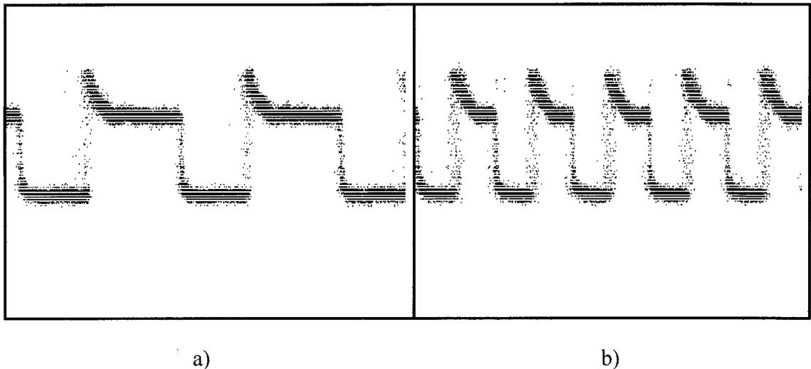
Figure 4-16: Square waveforms from the output of the optical receiver with a current mirror preamplifier at a) 100Mbps and b) 200Mbps.
