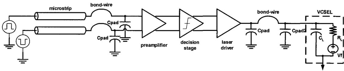
Figure 2-12: Block diagram of circuit used to simulate the optical transmitter.
