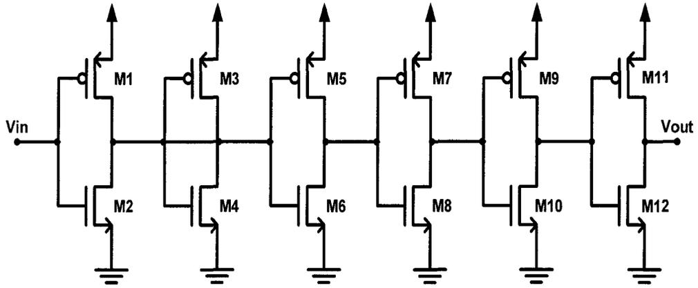
Figure 3-12: Schematic of the decision stage implemented for the optical receiver.
