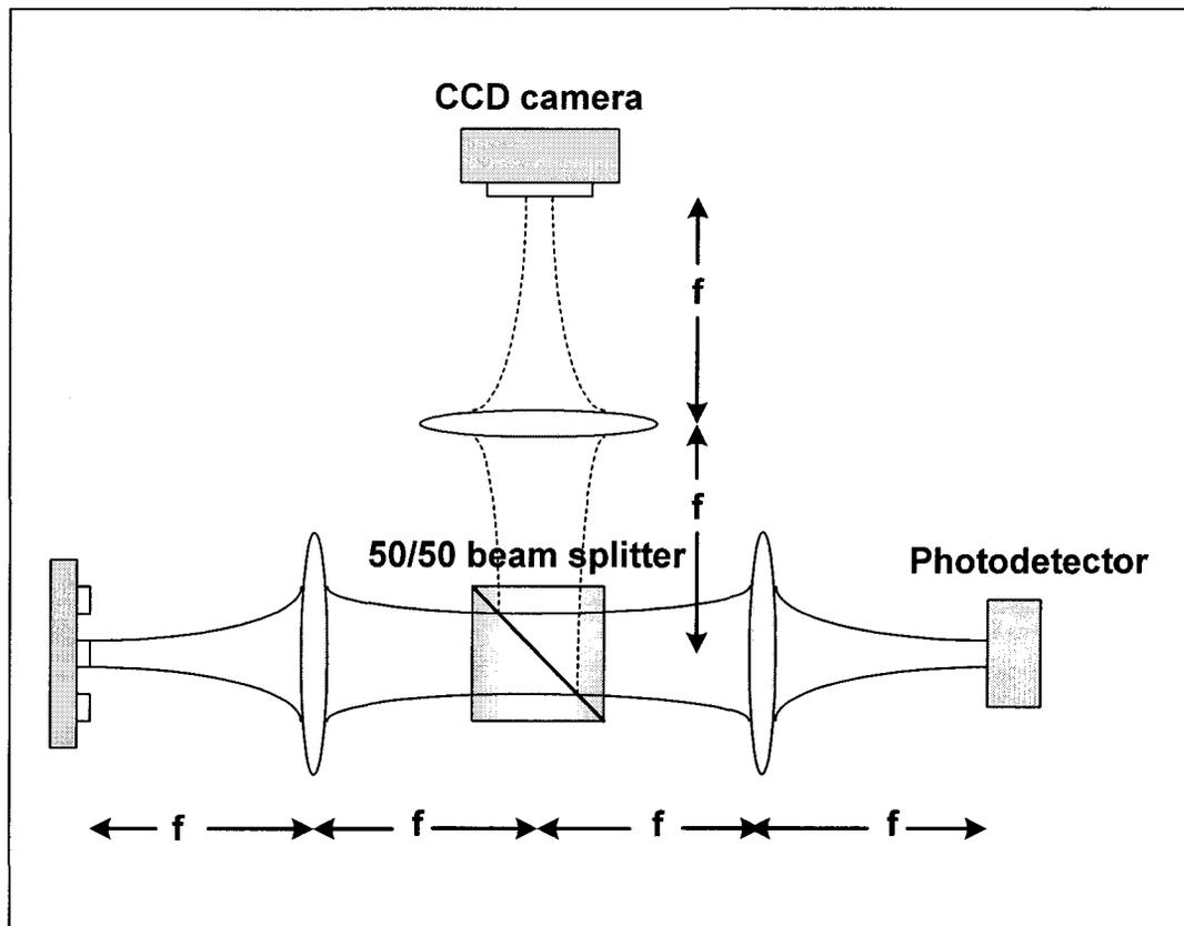
Figure 4-9: Block diagram of a telecentric optical relay system of the test setup for the optical transmitter.
