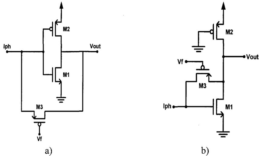
Figure 3-2: Examples of transimpedance amplifier with high input impedance.
