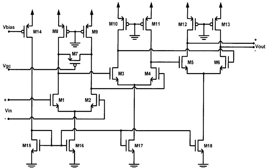
Figure 3-7: Schematic of the fully differential post-amplifier.
