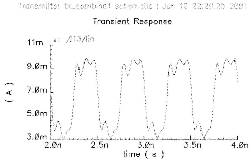
Figure 2-17: Transient response of the current provided to VCSEL by the push-pull laser driver, at 4Gbps.
