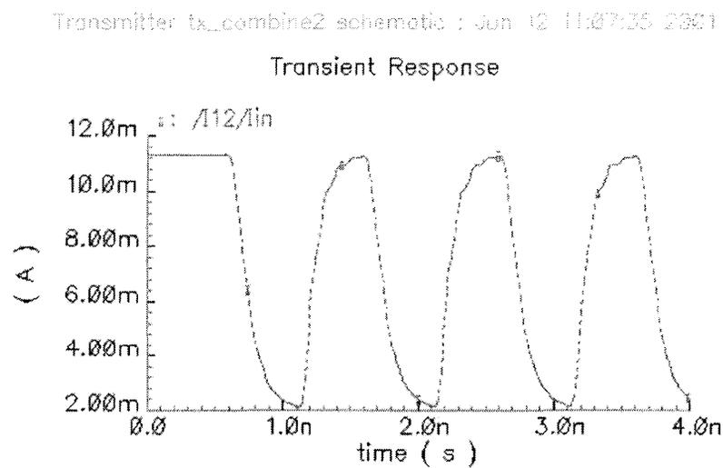
Figure 2-15: Transient response of the current provided to VCSEL by the fast-discharge laser driver, at 2Gbps.
