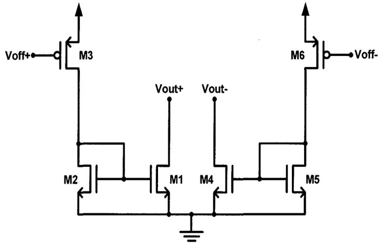
Figure 3-11: Schematic of an offset control circuitry.
