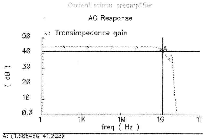
Figure 3-6: Frequency response of the current mirror preamplifier.
