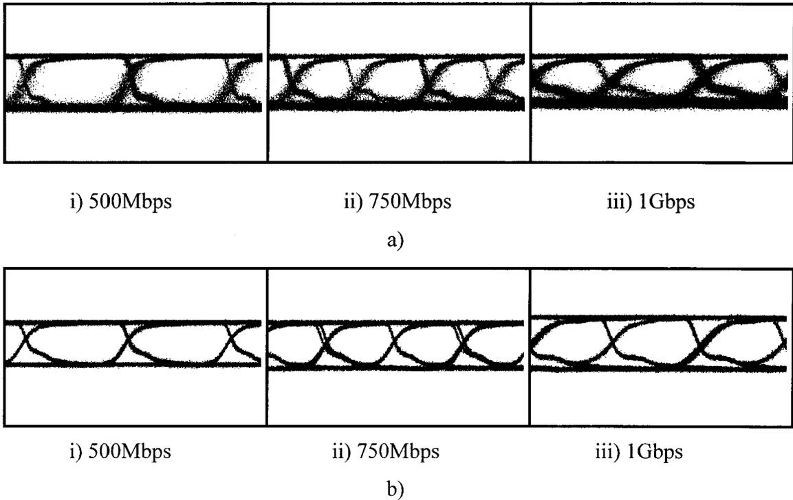
Figure 4-15: Eye patterns generated by the optical transmitter circuits with a) fast-discharge laser driver, b) push-pull laser driver using  $2^{32}-1$  PRBS.
