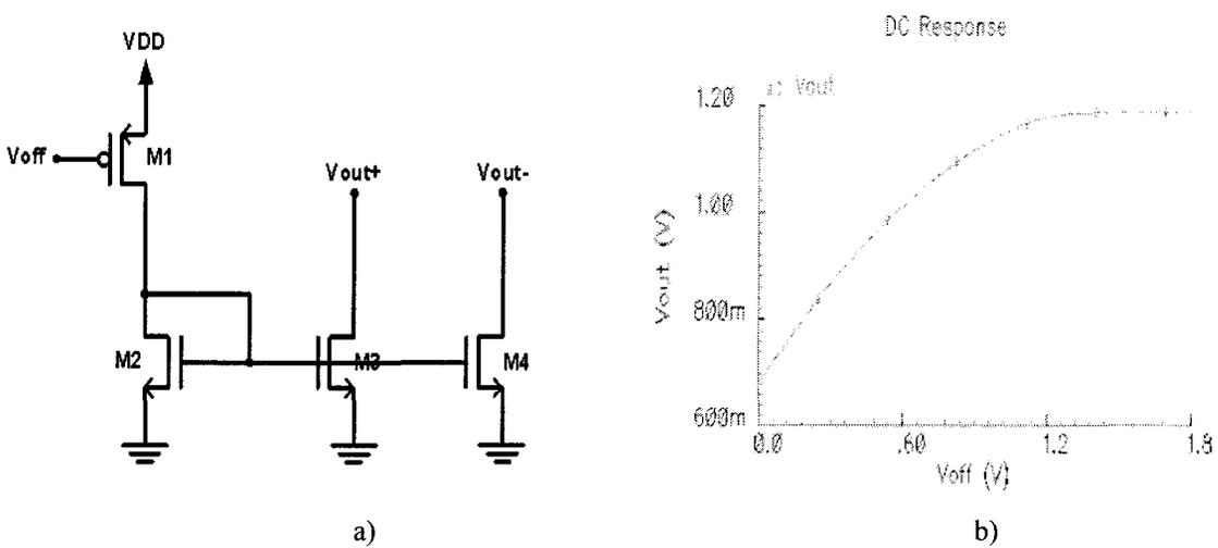
Figure 2-5: a) Schematic of an offset control circuit. b) The average output voltage of the preamplifier with respect to  $V_{off}$ .
