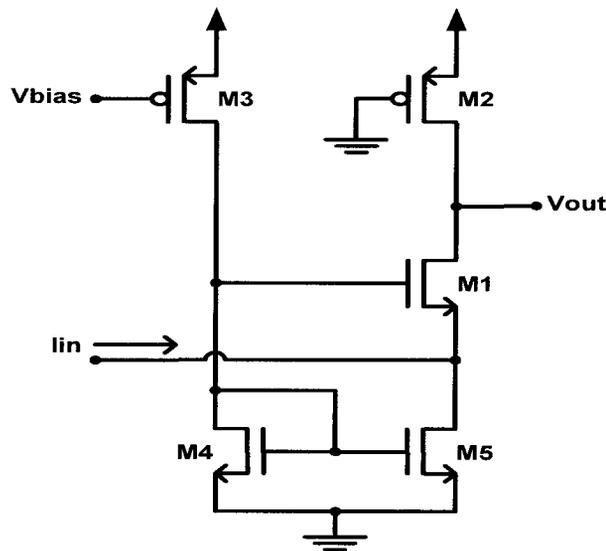
Figure 3-3: Schematic of a common gate preamplifier.
