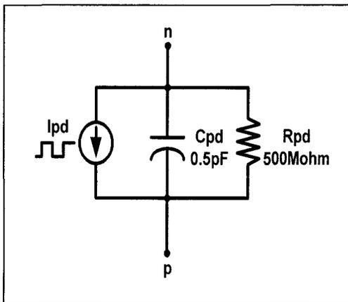
Figure 3-17: Circuit model of the photodiode used in optical receiver simulations.
