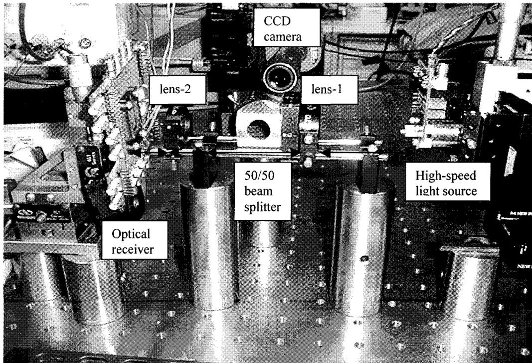
Figure 4-13: Photograph of the actual test setup to test the receiver chip.
