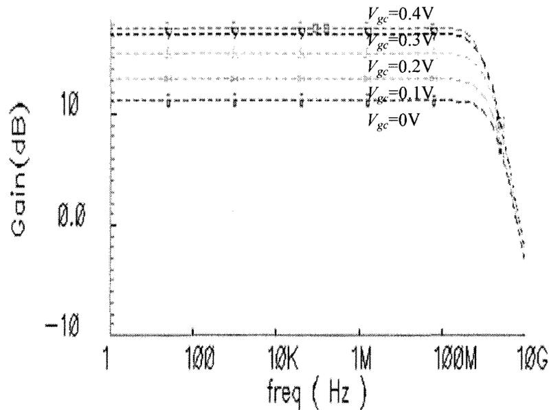
Figure 2-4: Frequency response of a GCFD amplifier due to different values of gain controlling voltage.
