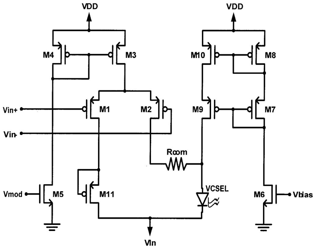
Figure 2-9: Schematic of a current steering laser driver.
