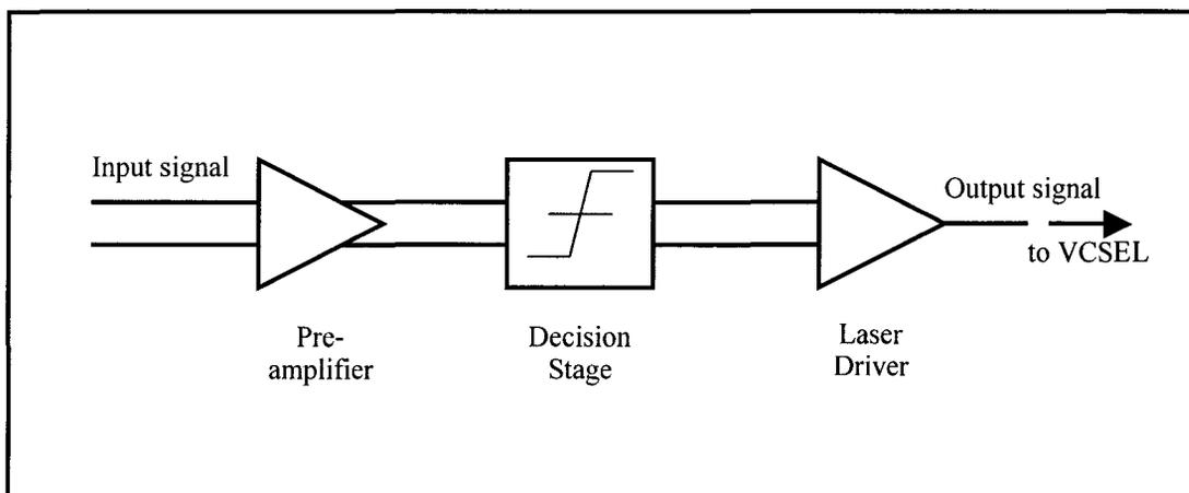
Figure 2-1: A block diagram showing the architecture of an optical transmitter circuitry.
