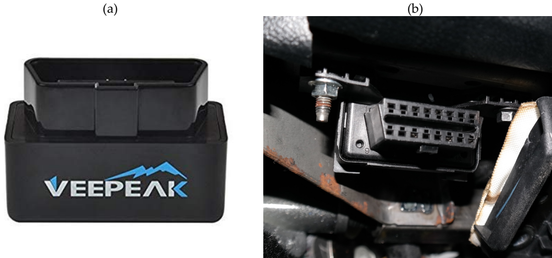
Figure 1: (a) Wireless OBD Scanner and (b) OBD-II port under the steering wheel
