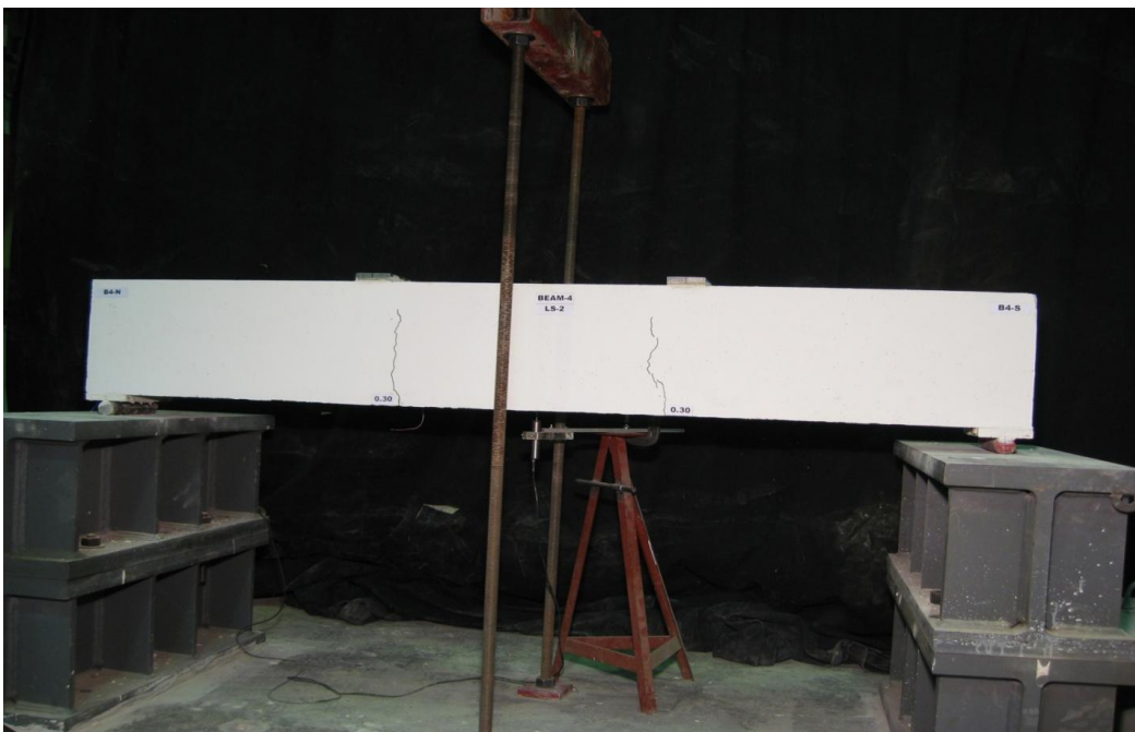
Figure D.28– Cracking pattern for beam 4 at a load of 30.2 kN (B4-LS2)
