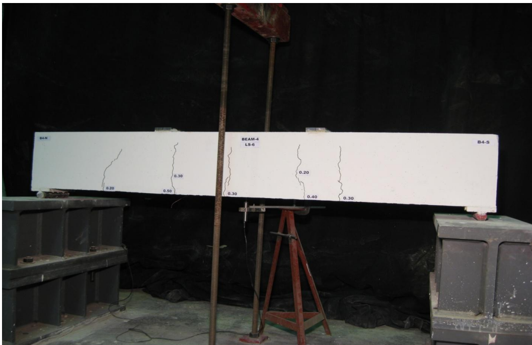
Figure D.32– Cracking pattern for beam 4 at a load of 49.51 kN (B4-LS6)
