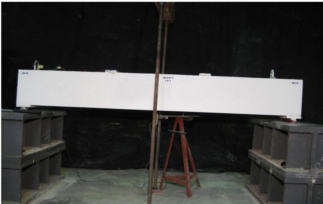
Figure D.38– Cracking pattern for beam 5 at a load of 20.45 kN (B5-LS1)
