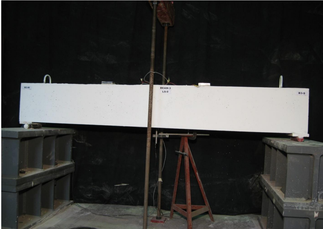
Figure D.13– Cracking pattern for beam 3 at zero load (B3-LS0)
