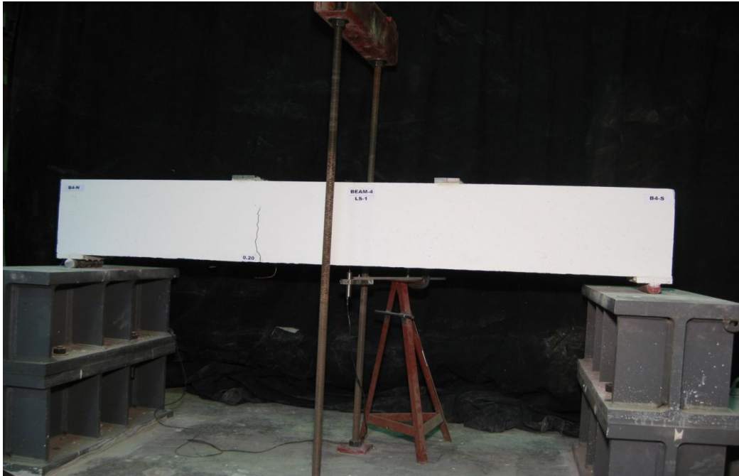
Figure D.27– Cracking pattern for beam 4 at a load of 25.23 kN (B4-LS1)
