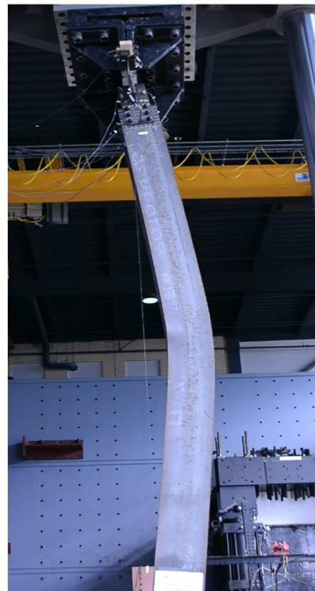
Figure 7 (a) gusset buckling in J360-REF; (b) overall minor-axis brace buckling in J310-REF
