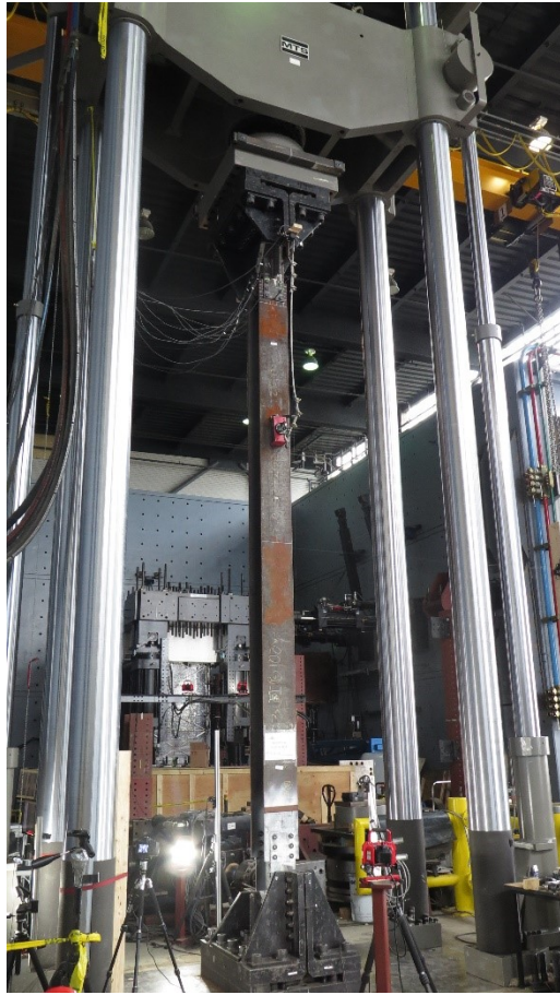
Figure 2 Test set-up of the full-scale I-shape brace and connection assembly [18,19]
