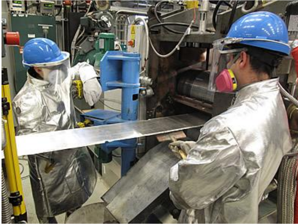
Fig. 3.1 TRC machine in operation at CANMET-MTL Hamilton, Ontario [3]
