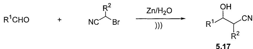
**Table 5.3 Zinc-Mediated Coupling Reaction of Bromoacetonitrile with Aldehyde in Water**
