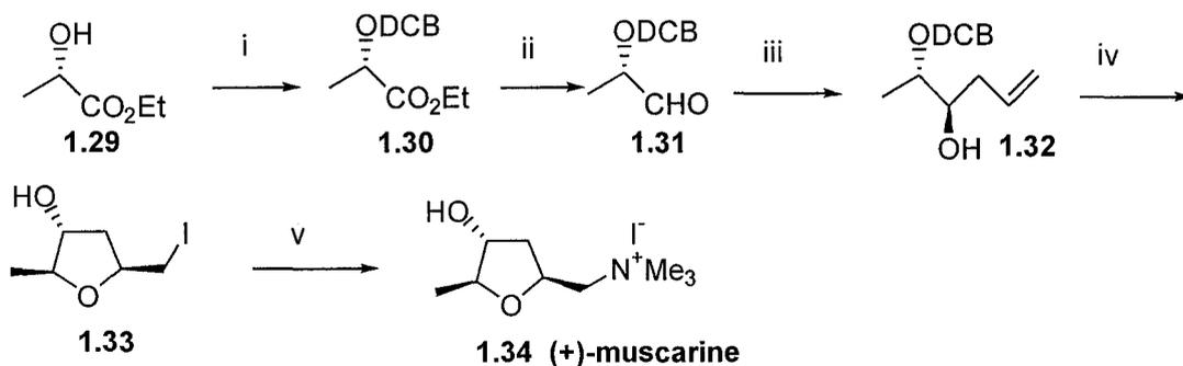
(i)  $DCBBBr/Ag_2O/Et_2O$ , reflux, 6h (ii)  $DIBAL-H/Et_2O$ ,  $-78^\circ C$ , 2h. (iii) Allylbromide/ $Zn/H_2O/NH_4Cl$ , 3h (iv)  $I_2/MeCN$ ,  $0^\circ C$ , 3h. (v)  $NMe_3/EtOH/80^\circ C/4h$
