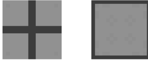
Figure 19: Prescribed regions of material (dark grey) to ensure connectivity between unit cells.
