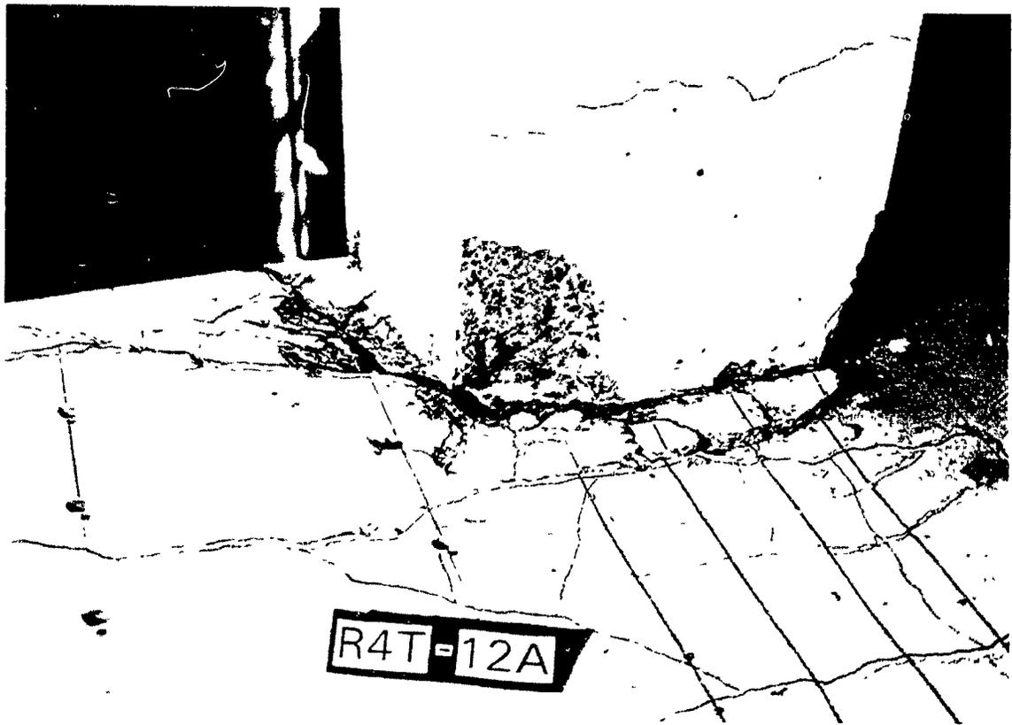
**Figure 3.18:** Cracking and crushing of concrete in slab for specimen R4T
