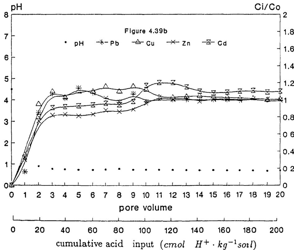
Figure 4.39 Breakthrough curves of pH and  $C_i/C_0$  of Pb, Cu, Zn, and Cd versus pore volume of kaolinite soil column when the columns were leached with (4.39a) low acidic permeant solution and (4.39b) high acidic permeant solution.
