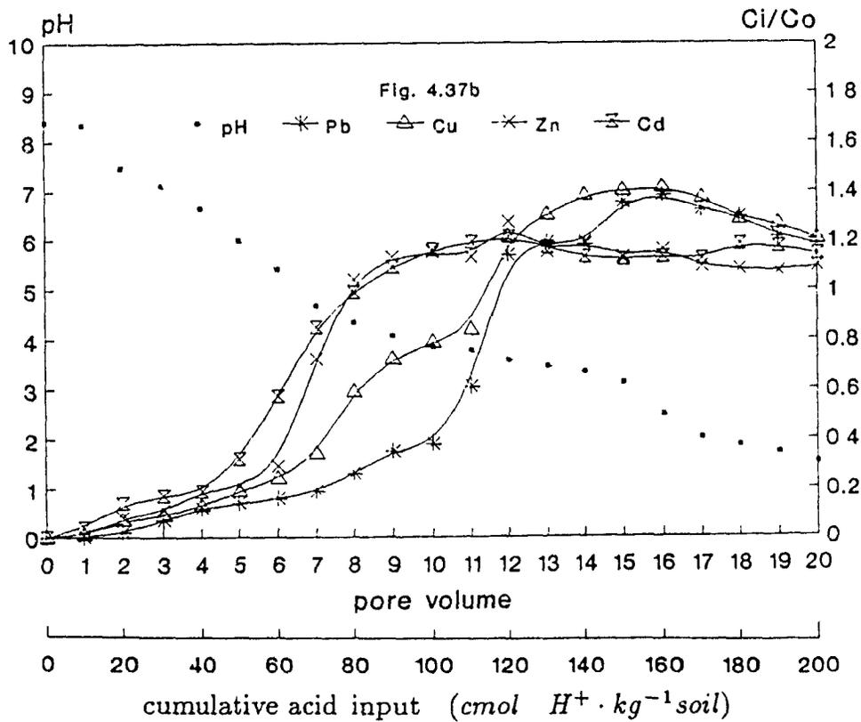
Figure 4.37 Breakthrough curves of pH and  $C_i/C_0$  of Pb, Cu, Zn, and Cd versus pore volume of illite soil column when the columns were leached with (4.37a) low acidic permeant solution and (4.37b) high acidic permeant solution.
