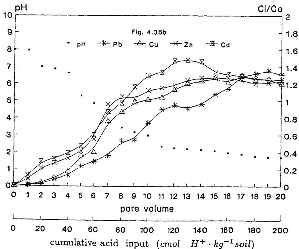
Figure 4.38 Breakthrough curves of pH and  $C_i/C_0$  of Pb, Cu, Zn, and Cd versus pore volume of natural clay soil column when the columns were leached with (4.38a) low acidic permeant solution and (4.38b) high acidic permeant solution.
