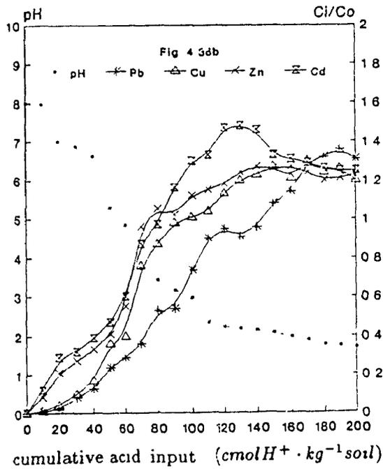
Figure 4.41 Comparison of the results from the soil suspension test and the soil column test of natural clay soil.
