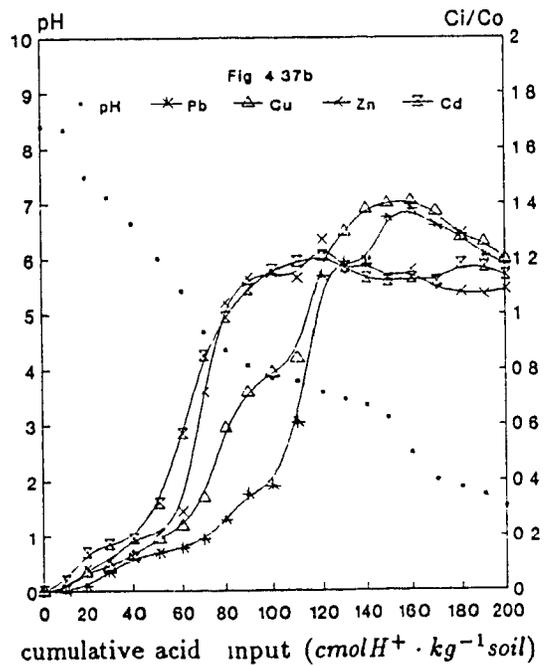
Figure 4.40 Comparison of the results from the soil suspension test and the soil column test of Illite.
