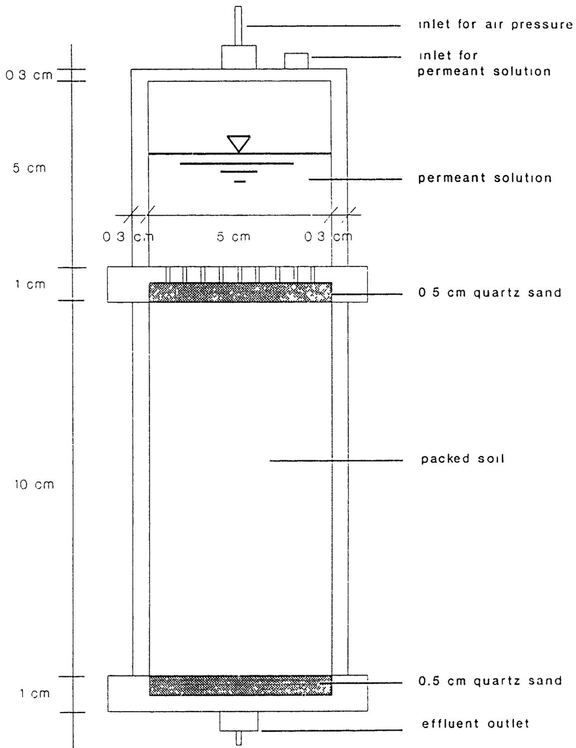
Figure 3.3 Schematic representation of a soil column used in this study
