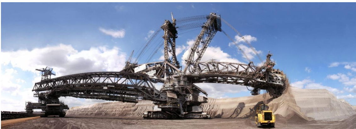
Figure 2. 3. Bagger 288 bucket-wheel excavator. From (Mining-Technology, 2018)
