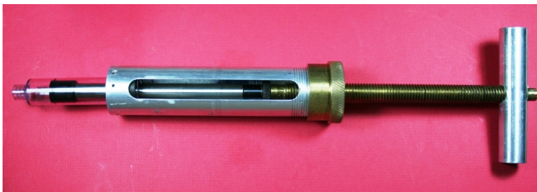
Figure 21: The entire injection setup, including the syringe, plunger and the device with a threaded rod and T-handle
