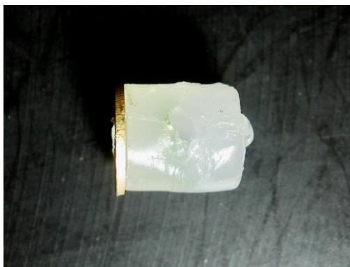
Figure 34: An example of an air bubble 3 mm in diameter entrapped in a cured gel sample excluded from further testing
