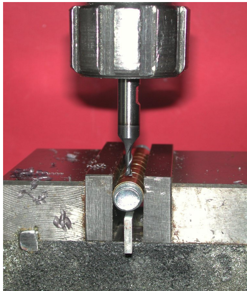
Figure 17: Slotting the thin brass tube with an end-mill of 7/64" width
