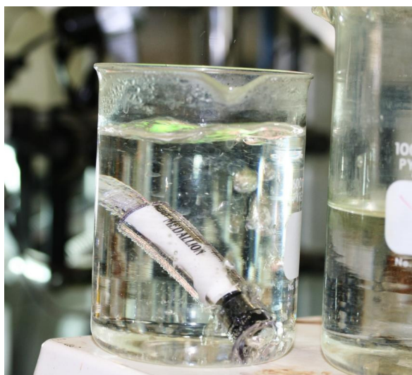
Figure 20: Hydrogel locked within a medallion 10 cc syringe, in boiling waterbath
