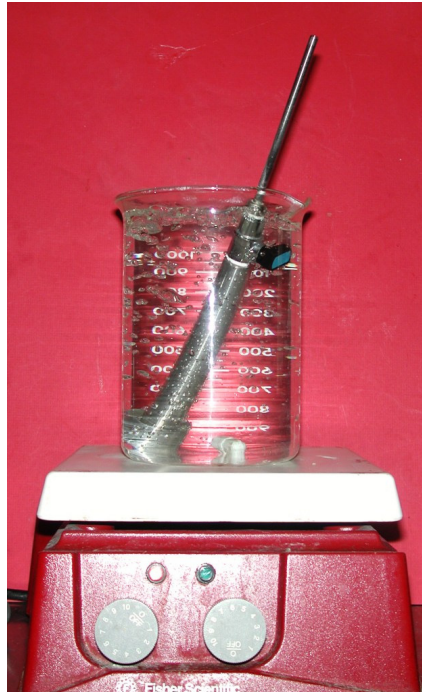
Figure 13: Boiling waterbath to melt the hydrogel encased in the syringe body
