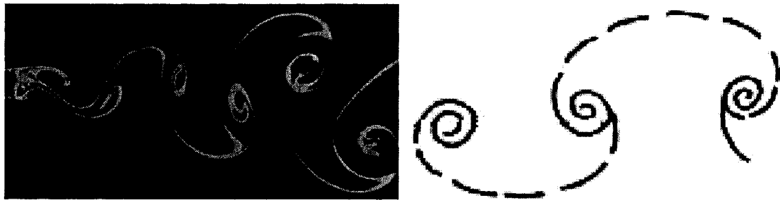
Figure 1-13 (left): Karman street [16]. Figure 1-14 (right): Reverse Karman street [17].
