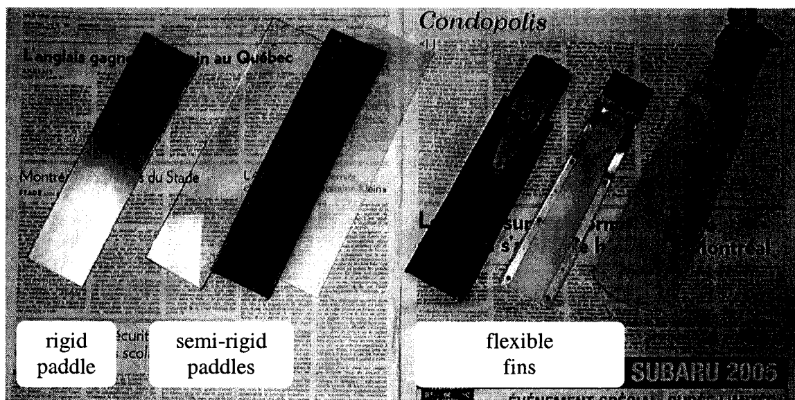
Figure 3-10: Rigid and semi-rigid paddles, and flexible fins. All paddles, except the rigid paddle, were developed by Shane Saunderson at the Ambulatory Robotics Laboratory.
