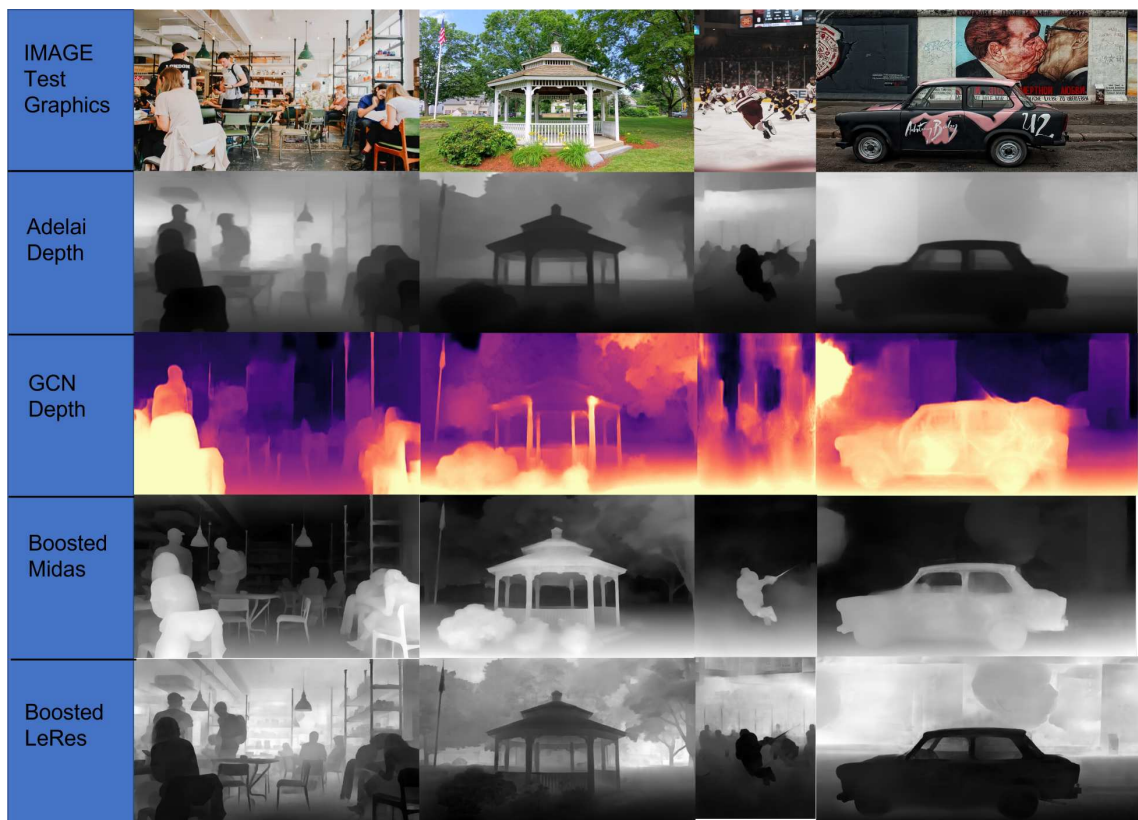
Fig. 3.2: Depth generation quality comparison across algorithms.
