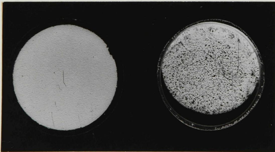
Fig. 6. Silver iodide samples prepared from methanol and ethanol suspensions respectively.
