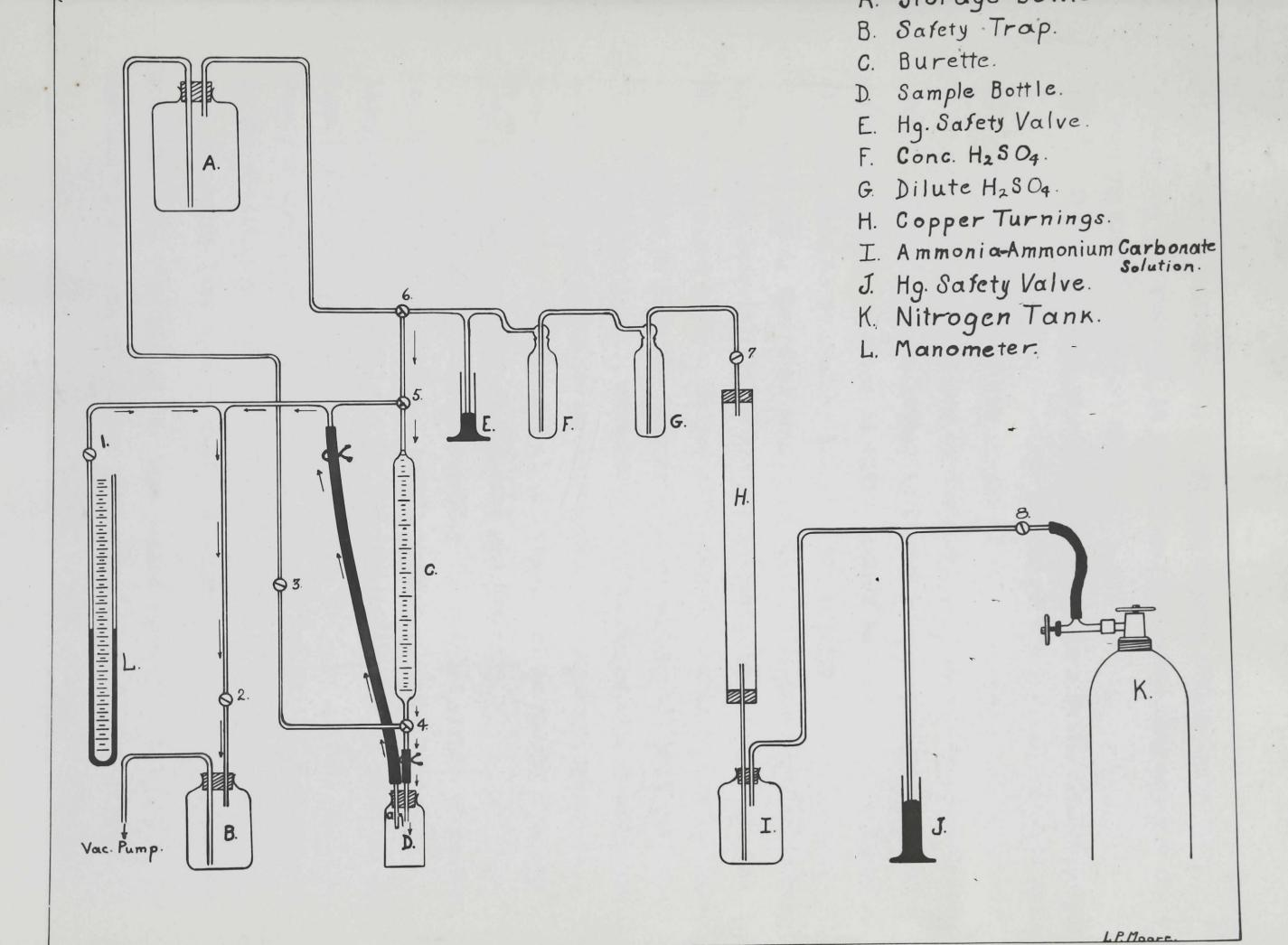
about 30 determinations. (E) & (J) are mercury safety traps to regulate the gas pressure in the system, (E) containing about 5 cm. of mercury and (J) somewhat more.
