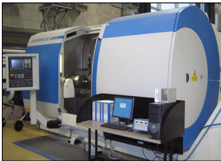
Figure 3-1 (b) Boehringer-NG200 CNC turning center used for turning tests
