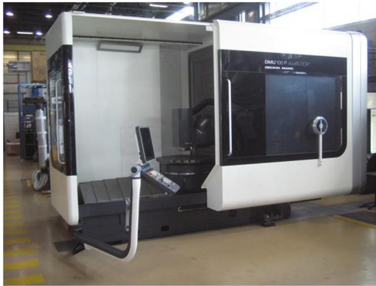
Figure 3-1 (a) DMU-100P duoBlock CNC machining center used for milling tests
