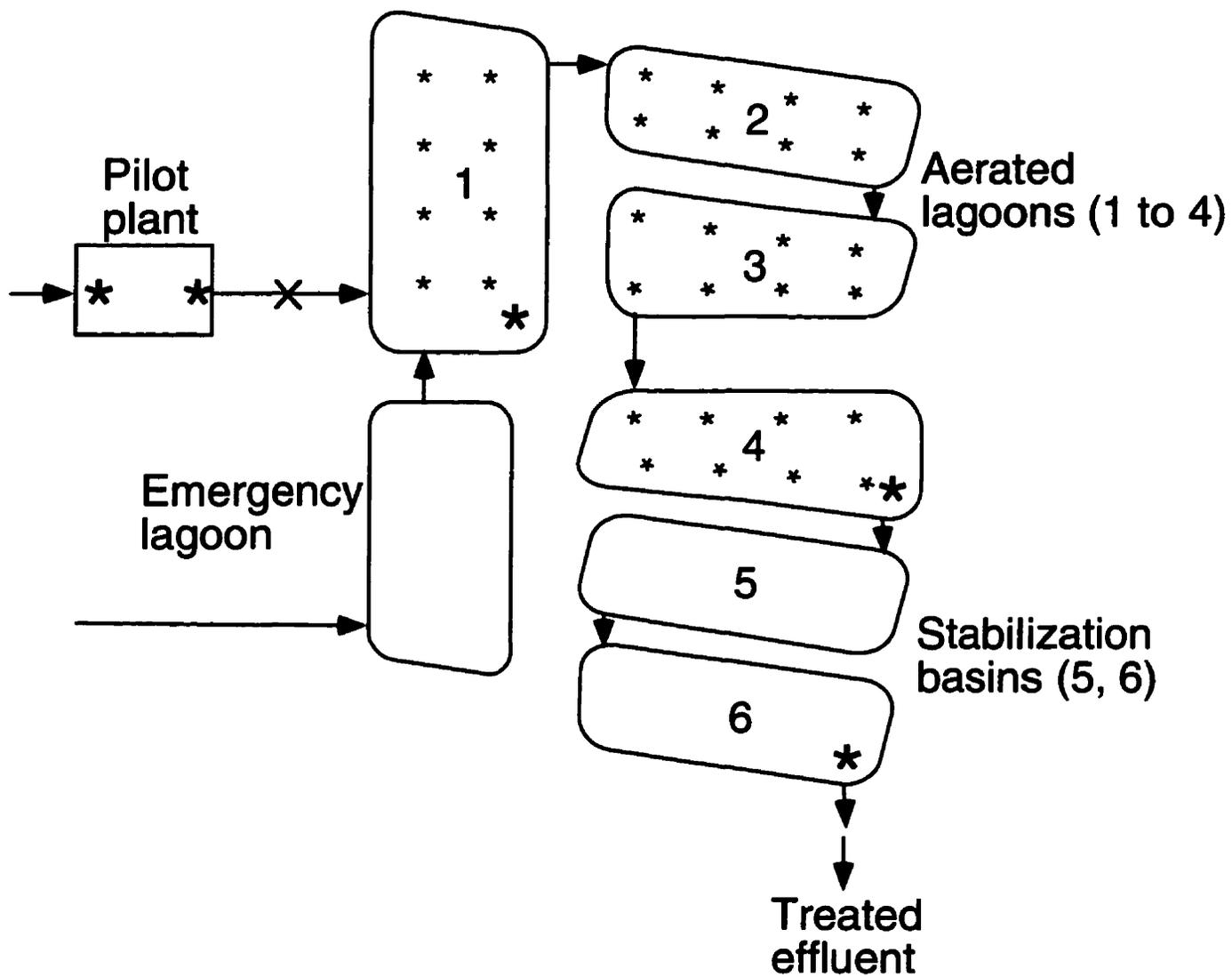
**Figure 25. Schematic of a kraft pulp and paper mill effluent treatment system and a pilot plant.** The stars indicate aerators(\*) or the sites from which water and sediment samples were collected (★).
