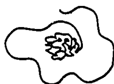
Figure 1.6. Structure of a monomolecular micelle formed by an AB block copolymer molecule in a nonsolvent for the B block. 18
