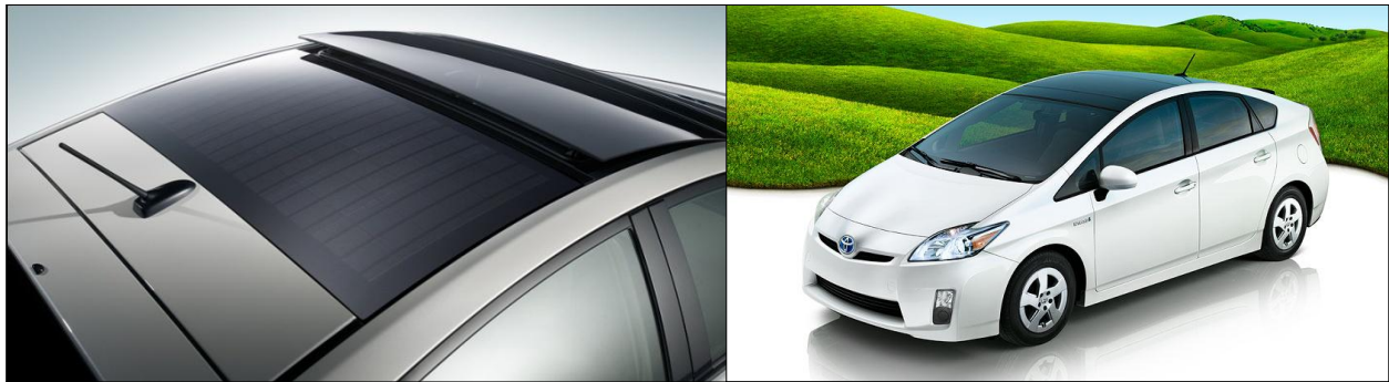
Figure 2-5. Toyota Prius - The first mass produced car with solar panels as the sunroof. Source : www.toyota.com/prius-hybrid
