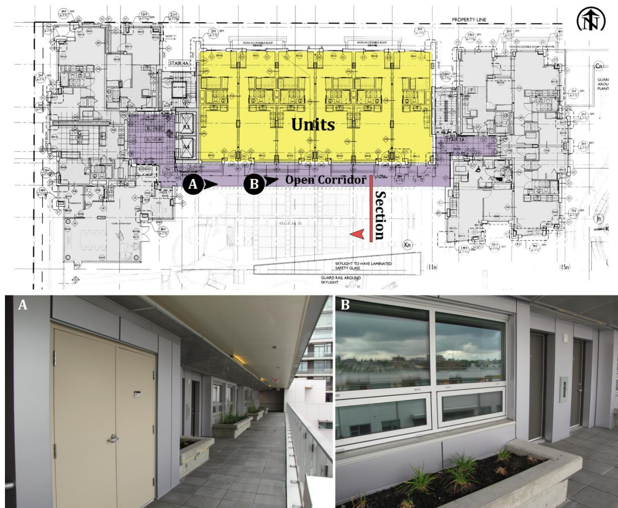
Figure 3-16. Open Corridor and its role in Passive Solar Design – Section f-f will be analysed in the Figure 3.18.
