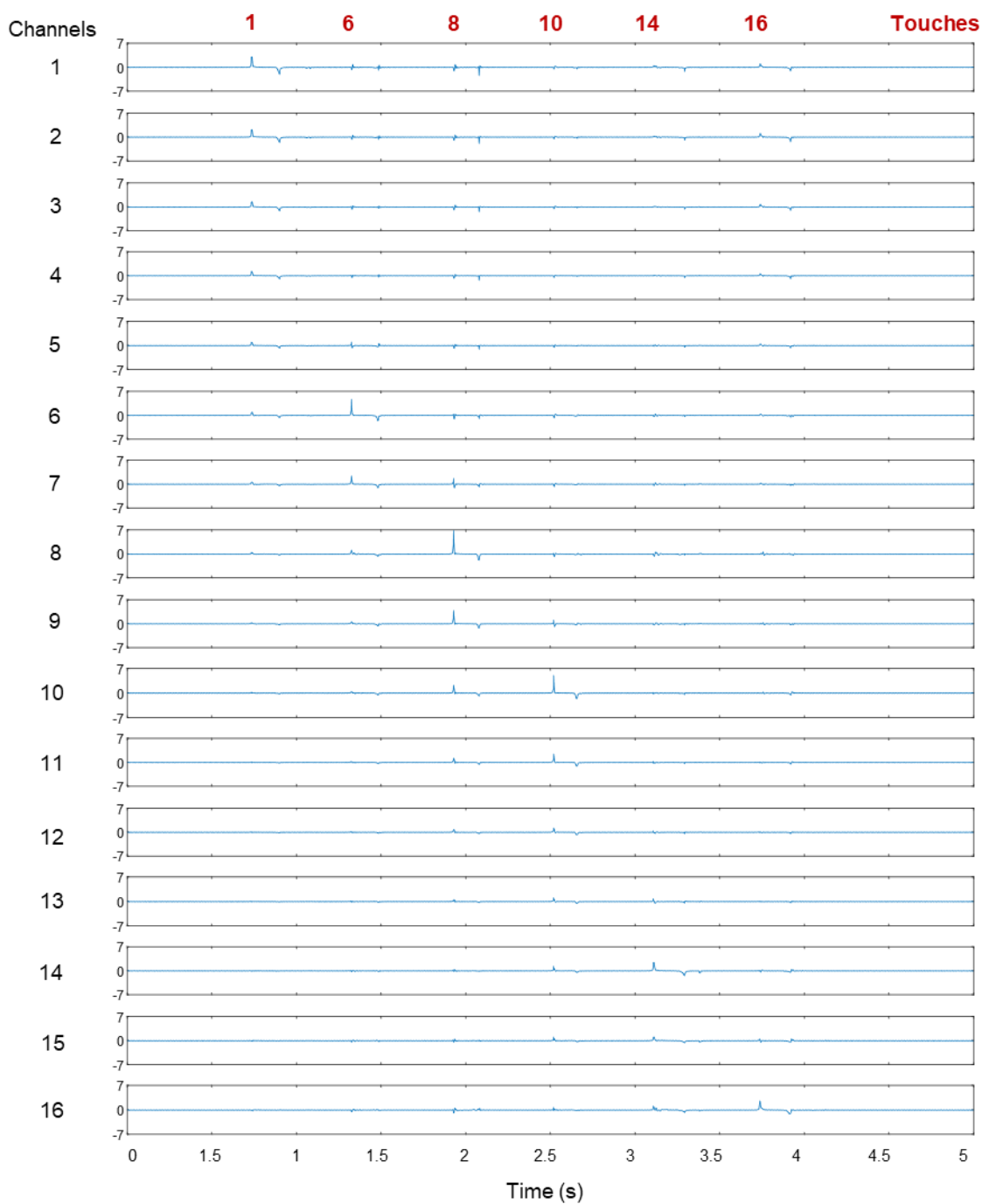
Figure 4.28. Raw output signals of all 16 channels during single-point touches on the ionic touchpad. The touched pixels in sequence were 1, 6, 8, 10, 14, and 16.
