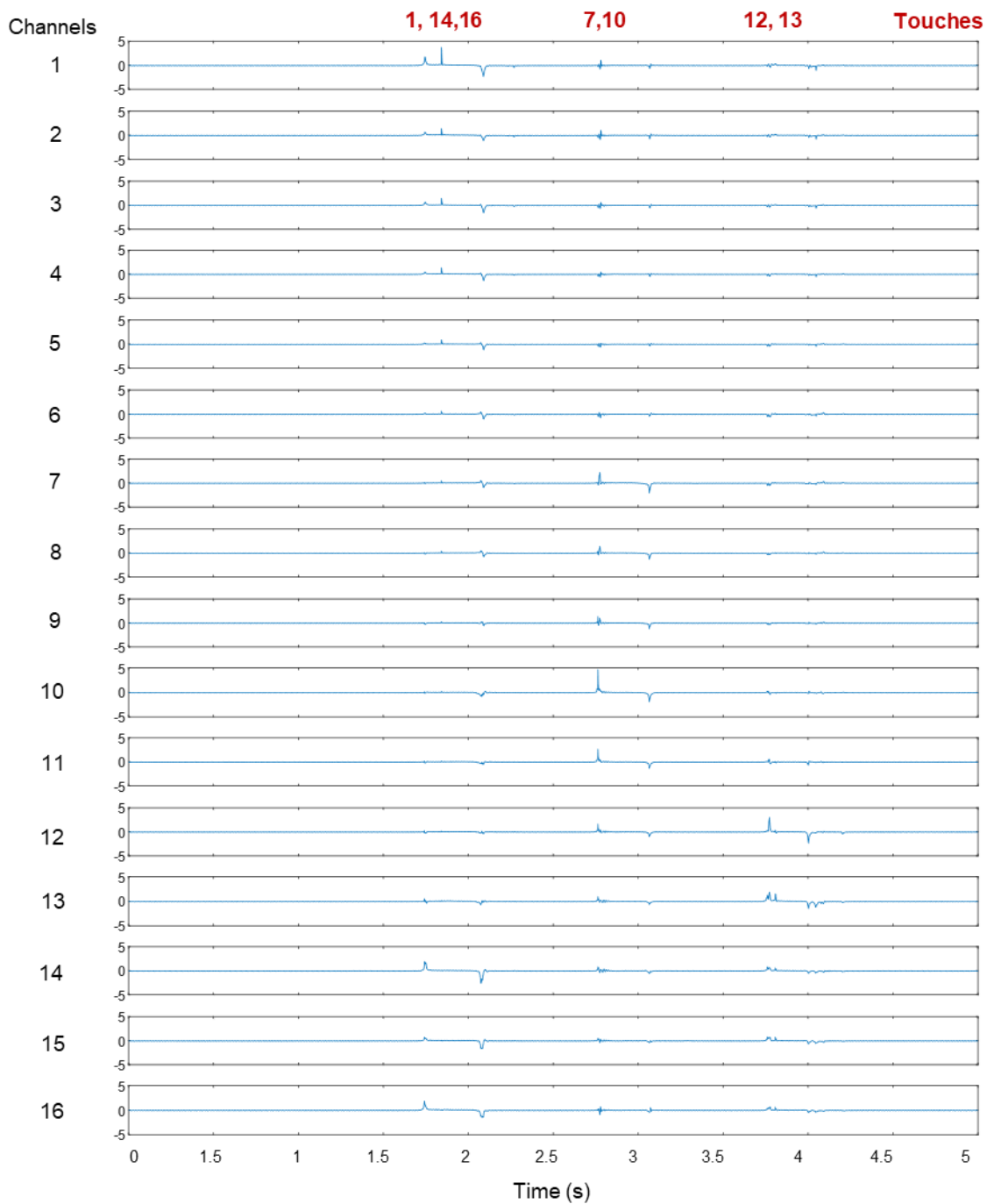
Figure 4.29. Raw output signals of all 16 channels during multi-point touches on the ionic touchpad. The touched pixels in sequence were 1, 14, 16; 7, 10; and 12, 13.
