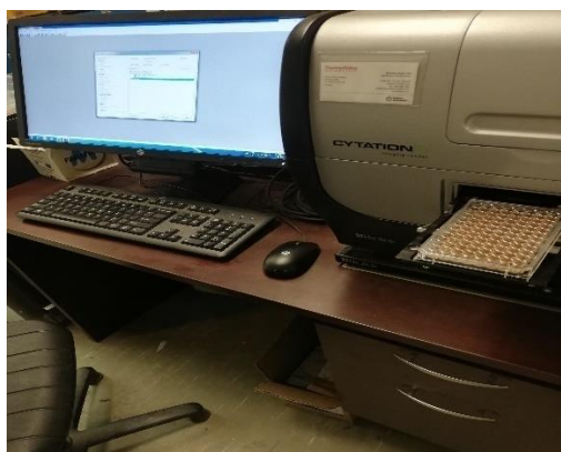
Figure 3.1: The Cytation instrument connected to a computer.
