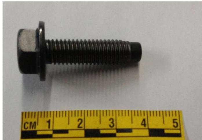
Figure 4.1: Hex flange head screw sample.
