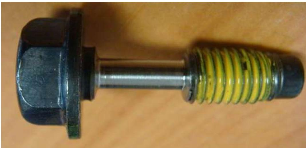
Figure 4.4: Machined tensile sample – modified ASTM E8-13a Fig. 8 Specimen 4.
