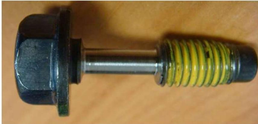
Figure 6.7: Machined tensile sample – modified ASTM E8-13a (Standard Test Methods for Tension Testing of Metallic Materials) [5] Fig. 8 Specimen 4
