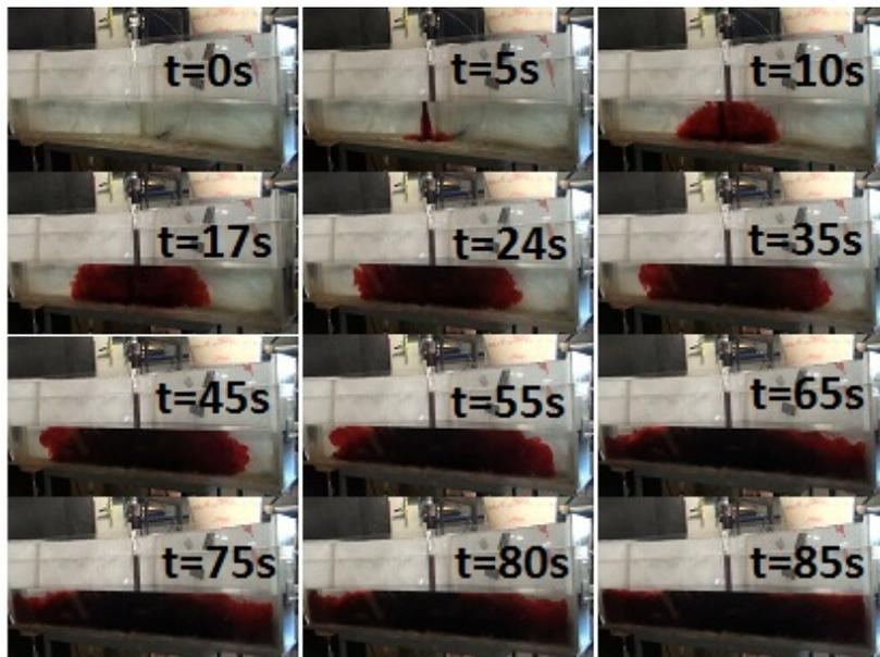
*Figure-6.7(b) Tracer dispersion under an aligned shroud condition*
