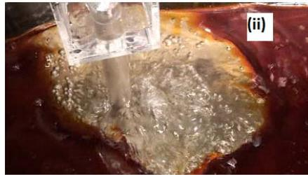
*Figure-6.8(a) Exposed 'eye' with a biased shroud (i) 4% (ii) 6% gas injection by volume*
