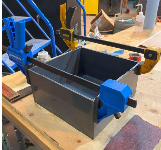
Figure 7. The constructed reservoir made of PVC was clamped as the cement dried.
