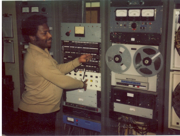
Figure 13: Manuel Fitch adjusts a patchbay connection at a WJLD equipment rack, with the automation system's cartridge carousel visible to the right. Courtesy of the Birmingham Black Radio Museum.
