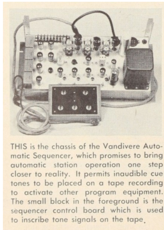
Figure 3: The Vandivere Automatic Sequencer, as shown in Broadcasting · Telecasting . A caption reads, “This is the chassis of the Vandivere Automatic Sequencer, which promises to bring automatic station operation one step closer to reality. It permits inaudible cue tones to be placed on a tape recording to activate other program equipment. The small block in the foreground is the sequencer control board which is used to inscribe tone signals on the tape.” Scan courtesy of the Media History Digital Library.
