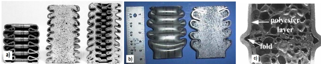
Figure 2.19: Progressive collapse for a) hollow and Al-foam-filled steel tubes, Seitzberger et al. b) Al-foam-filled tubes, Fraunhofer-USA report 1 and c) Al-foam at the location of tube instability, Toksoy et al. [63]
