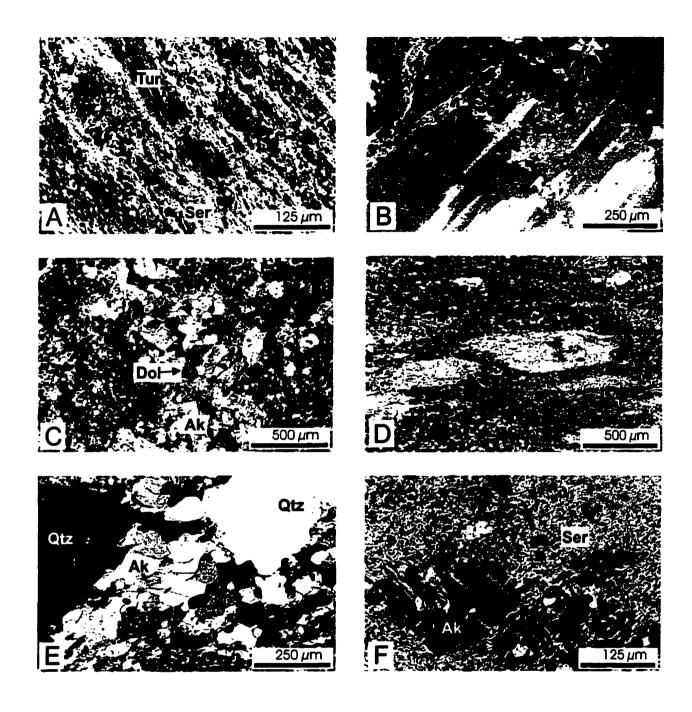
Figure 6: Alteration mineral paragenesis of the Ryne and Hourglass showings.
