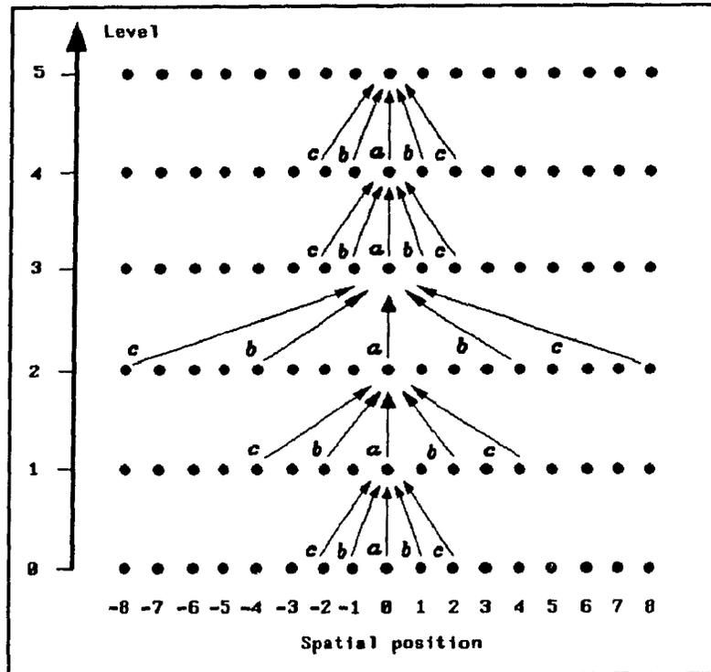
**Figure 3.8** Construction of a "hybrid" HDC. An expanding sampling rate of  $2^l$  is used up to a level  $l^*$  ( $= 3$ , for example) to obtain HDC levels to rapidly reach a given smoothing scale  $\sigma^*$  ( $> \sigma_3$ , in this example). Then a fixed sampling rate of 1 is used to produce HDC levels possessing smoothing scales around this  $\sigma^*$ .
