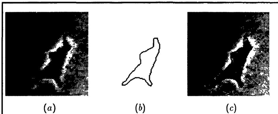
**Figure 1.4** Image segmentation using the snake. In (a) is shown the original intensity image. In (b) is shown the line drawing obtained from the optimal snake position. In (c), the snake in (b) is superimposed on the image in (a).
