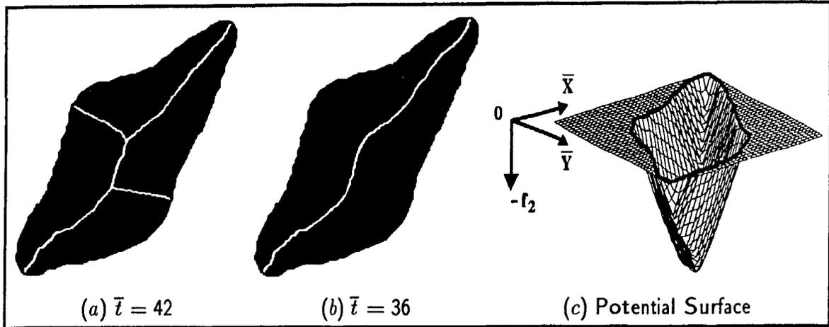
**Figure 5.6** Skeletons obtained from grassfire propagation combined with positive curvature extrema extraction at two different scales. In (a) the four most significant  $C$ 's were retained. In (b) only the two most significant  $C$ 's were retained. In the latter case, a stable state is reached earlier because the fire fronts are simpler. Time  $\bar{t}$  corresponds to iteration.
