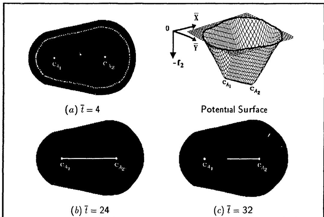
**Figure 5.7** Example of fire propagation on a shape made of two circular arcs joined by straight lines.  $C_{A1}$  and  $C_{A2}$  are the centers of the arcs. In the neighborhood of  $C_{A1}$  the ridge is made of increasing absolute distance values as shown by the potential surface. If the snake is attached at  $C_{A1}$  the true skeleton is obtained as shown in (b). Otherwise, the snake shrinks as shown in (c).
