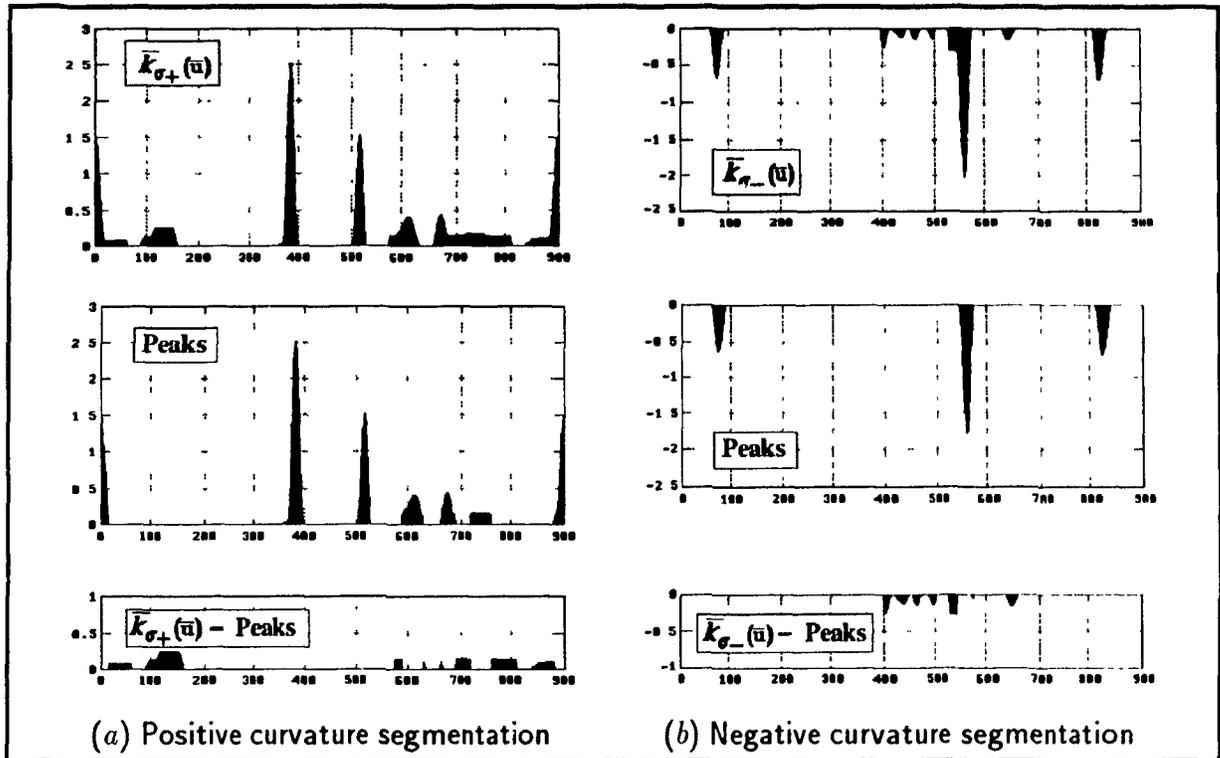
Figure 4.14 Segmentation of the curvature signal
