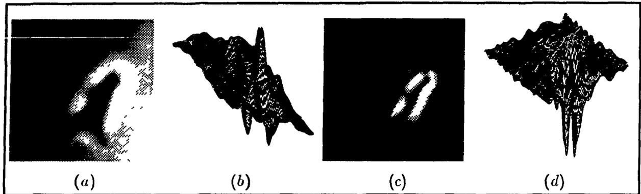
**Figure 1.3** Intensity image seen as a topographic map This three-dimensional (3-D) surface representation is produced by taking the intensity values as heights. White is considered the zero level height, while black is the highest level. In (a) is shown the image of a cell blurred using a Gaussian filter. In (b) is shown its representation as a 3-D surface. In (c) is shown the gradient of the image in (a), and in (d) is shown its representation as a 3-D surface.
