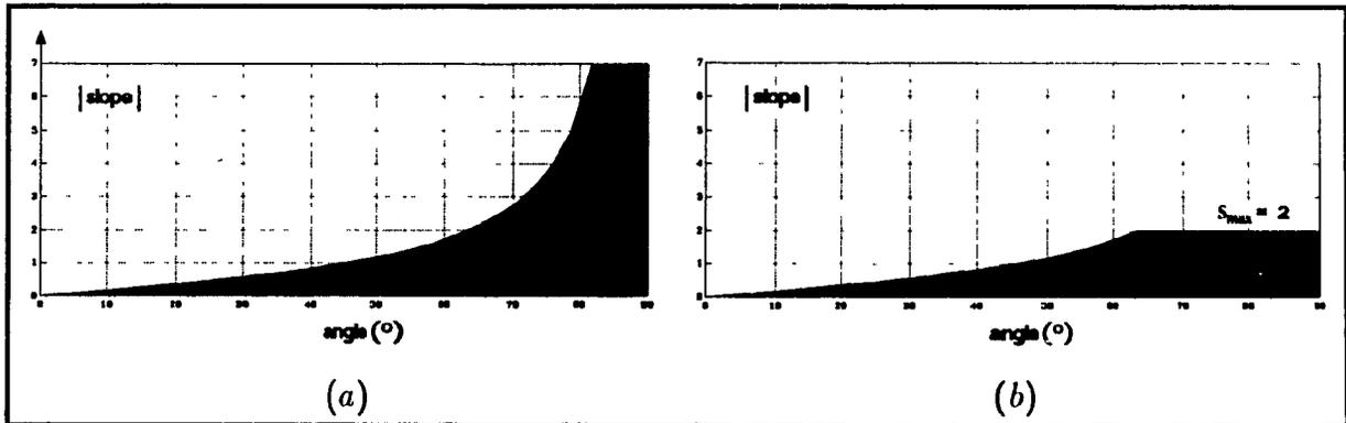
**Figure 2.4** The slope-amplitude problem. In (a) is shown the absolute values of the slope function. This function is asymptotic to infinity at an angle of  $90^\circ$ . In (b) is shown the clipped version of this function for  $S_{max} = 2$ .
