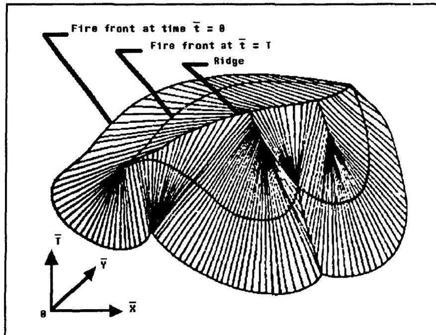
**Figure 5.1** 2-D dynamic grassfire, where the vertical coordinate represents time or distance from the ground state. The maximal directional slope of the obtained surface, which is the reciprocal of the grassfire velocity, is everywhere one except at the symmetric axis locus (ridges), where it is undefined. Adapted from [Blum73a], Figure 11
