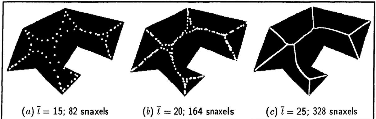
**Figure 5.12** Example of a grassfire propagation in three stages, with an increasing number of snaxels. In (a), a first coarse solution is obtained after 15 iterations. In (b), a more refined solution is then rapidly obtained by increasing the number of snaxels. In (c) is shown the final result for a continuous snake.
