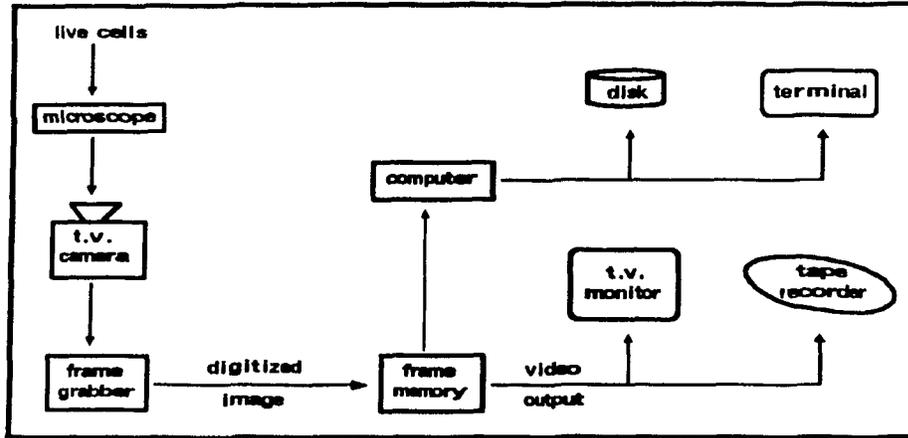
**Figure 3.2** Laboratory set-up consisting of a computerized video recording system. First, an analog image is obtained from a phase-contrast microscope using a t.v. camera. Then, the image is digitized using the frame grabber. Motion sequences are recorded, on disk or on tape, using the time-lapsed video technique. Adapted from [Noble86], Figure 7, Chapter 4, p. 57.
