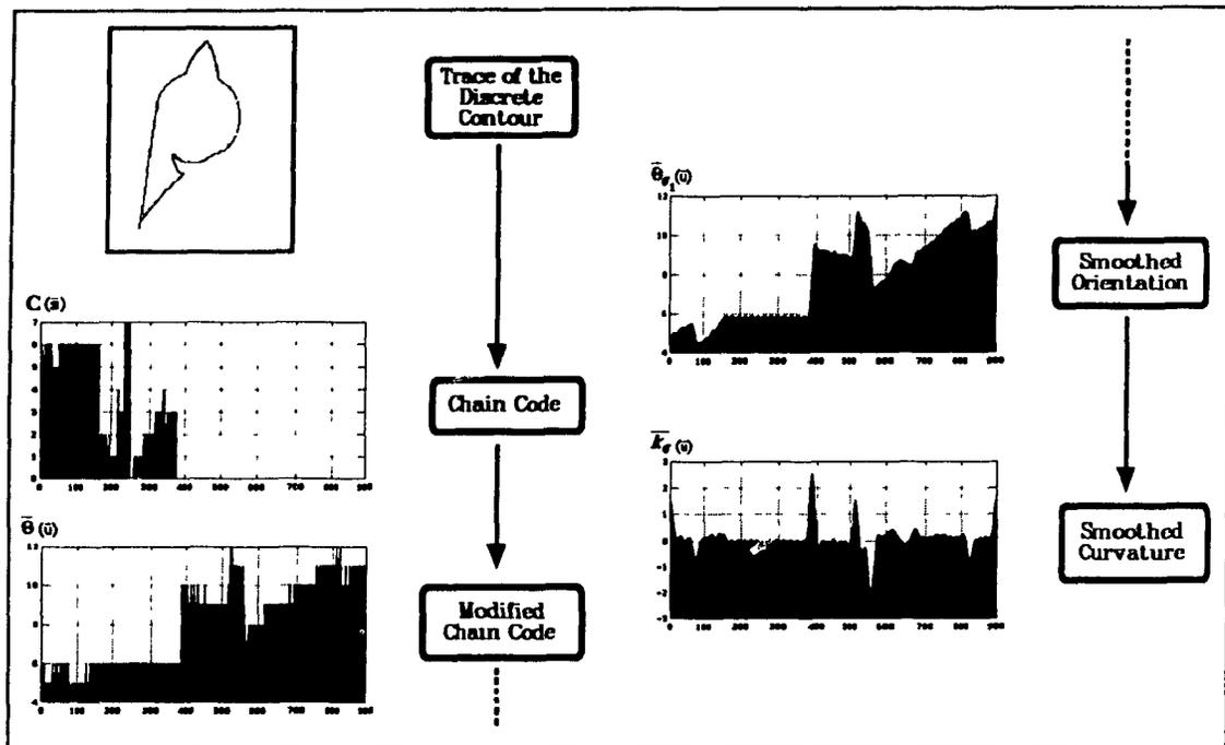
**Figure 4.4** From the trace of the discrete contour to smoothed orientation and curvature representations. The object shown in here and its discrete smoothed curvature  $\bar{k}_{\sigma}(\bar{u})$  will be used throughout this chapter to illustrate the complete curvature morphology approach.
