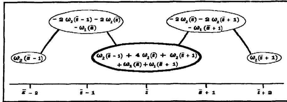
**Figure A.3** The nodal equation obtained by molecular summation of both the composite string molecule and the composite rod molecule
