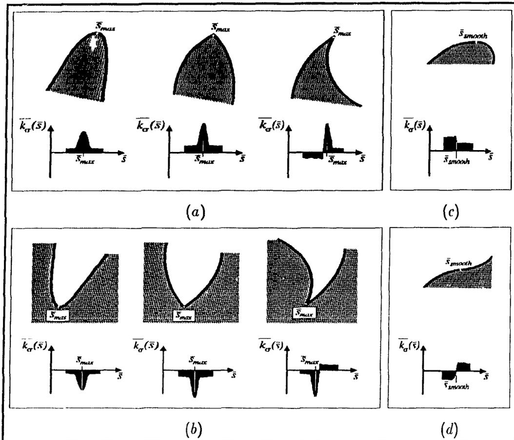
**Figure 4.1** Some curvature features and their contour counterparts in the discrete domain (a) protrusion, (b) depression, (c) smooth-join of the first type, (d) smooth-join of the second type. Only segments of a contour are shown. Contour pixels are traversed in a fixed counterclockwise direction. Therefore, the interior of the object delimited by the contour is defined as being to the left of the traversal direction (shaded area).
