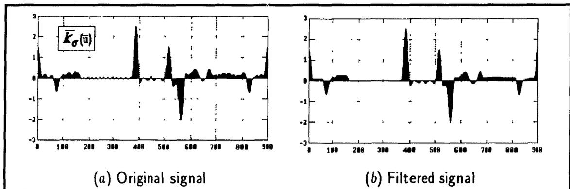
Figure 4.13 Example of removing noise from  $\bar{k}_{\sigma}$  using the hat transforms and the MCS
