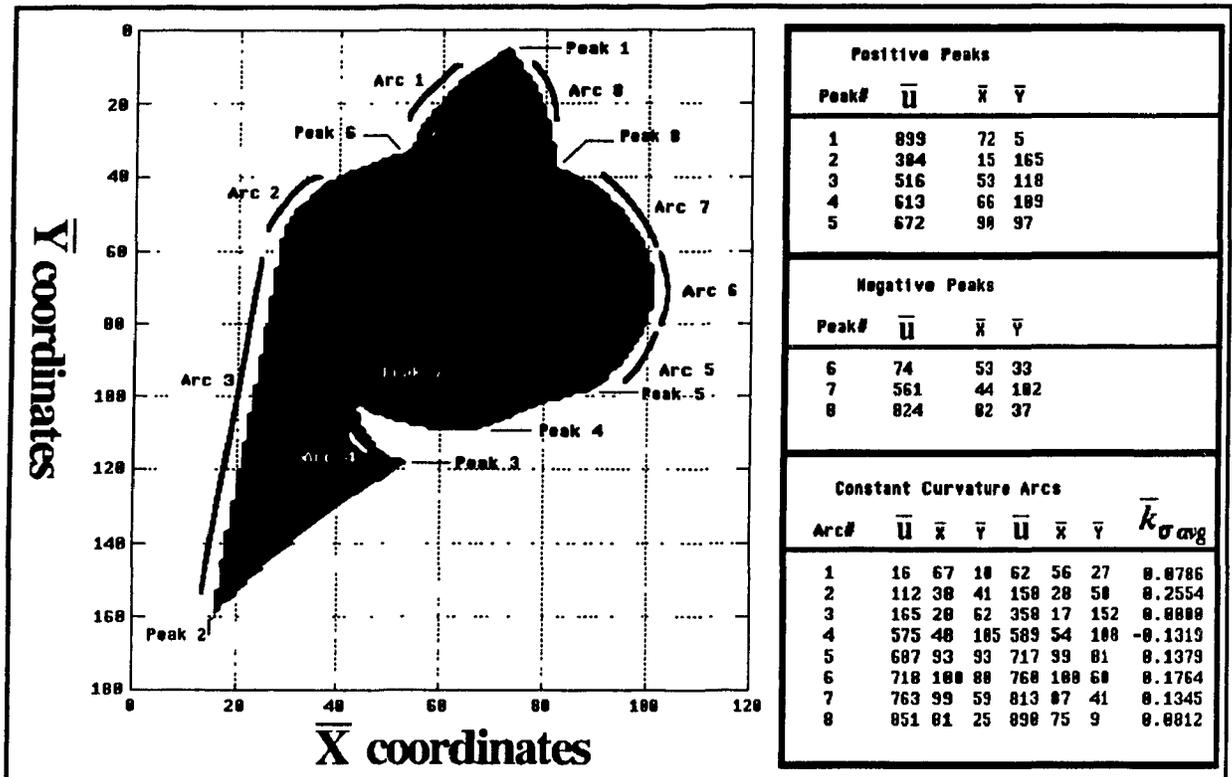
Figure 4.15 Contour segmentation based on the previously extracted curvature features
