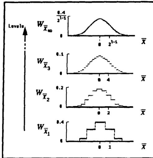
**Figure 3.4** Equivalent 1-D weighting functions (here  $W_{\bar{x}_l}$ , along the  $\bar{x}$  axis) converging to a 1-D Gaussian kernel (adapted from [Burt81], Figure 2)
