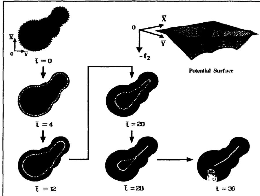
**Figure 1.7** Simulating the grassfire transform (i.e., shape skeletonization) using the snake model. The potential surface is shown at the top right corner. The fire is ignited at time  $\bar{t} = 0$  where time corresponds to iteration. The stable state occurs at  $\bar{t} = 36$  iterations. This last picture shows the final result when the number of snake elements is increased so that the snake is spatially connected, that is, without any gaps.
