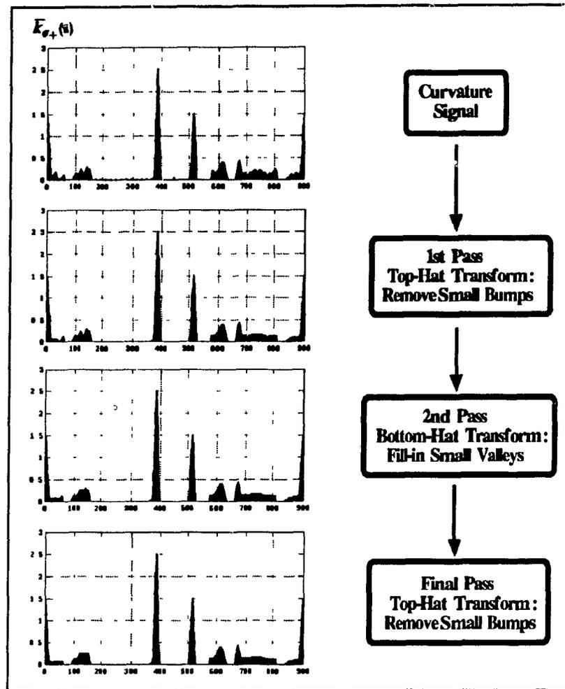
Figure 4.12 Removing noise from  $\bar{k}_{\sigma+}(\bar{u})$ . At each one of the three passes, the MCS is used to extract small bumps and depressions
