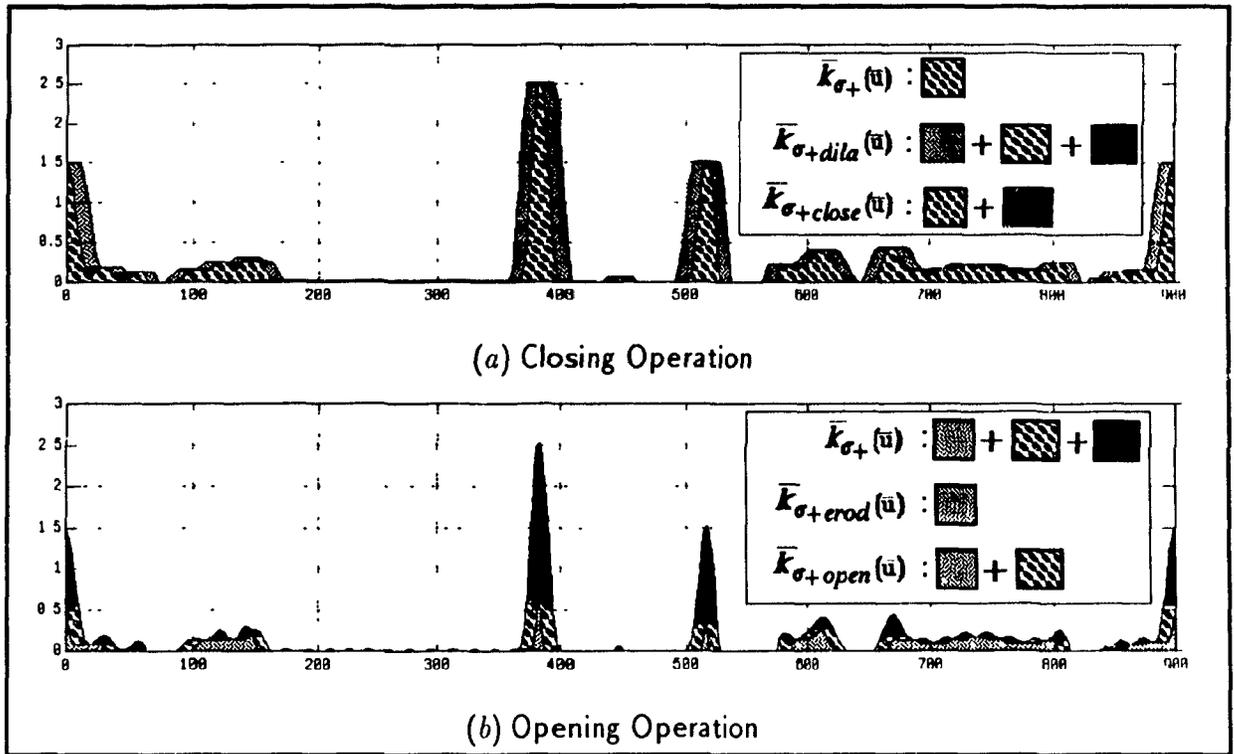
**Figure 4.7** Examples of closing and opening operations applied on a positive curvature function for a structural element of fixed width (here 21 arc length units wide)
