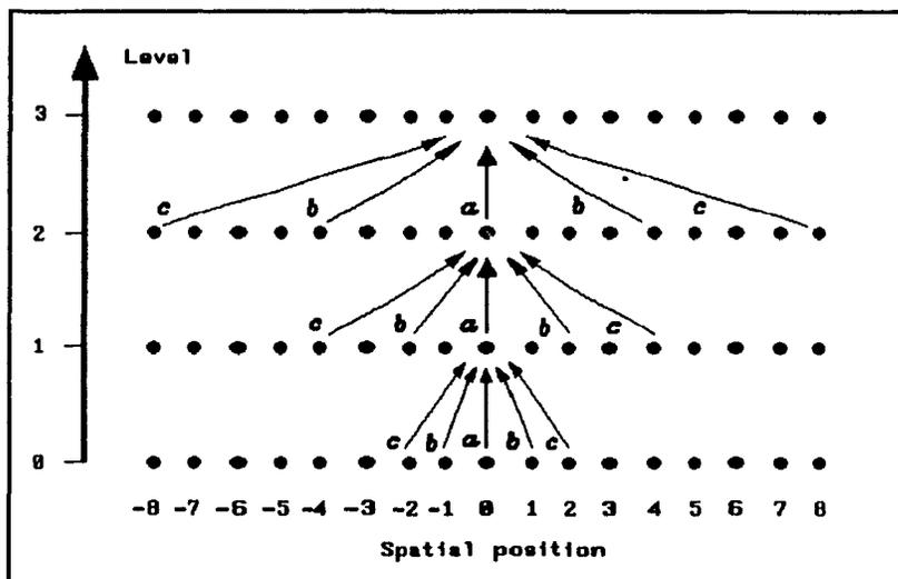
**Figure 3.5** A sketched representation of the HDC method (1-D case). The letters  $a$ ,  $b$  and  $c$  represent the weights of a mask ( $w_{\bar{x}}$  or  $w_{\bar{y}}$ ) of length five. The arrows represent the neighborhood relations from level to level of this recursive filtering method (i.e., how one level is built from the preceding one). Here nodes represent sample points of the HDC image. Adapted from [Burt81], Figure 1.
