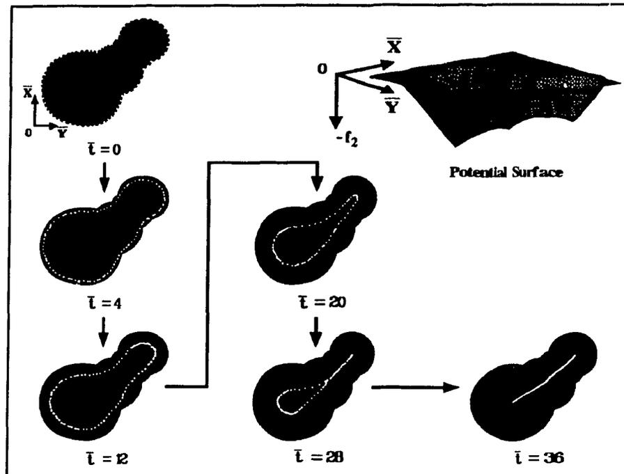
**Figure 5.3** Example of grassfire propagation on a blob-like shape. The potential surface is shown at the top right corner. The dark lines superimposed on it represent the snake at its initial and final states. The fire is ignited at time  $\bar{t} = 0$  where time corresponds to iteration. The stable state occurs at  $\bar{t} = 36$  iterations. This last picture shows the final result when the number of snaxels is increased so that the snake is spatially connected, that is, without any gaps.
