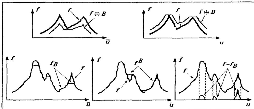
**Figure C.1** Examples of the four morphological operations and of the top-hat transform (adapted from [Serra82])
