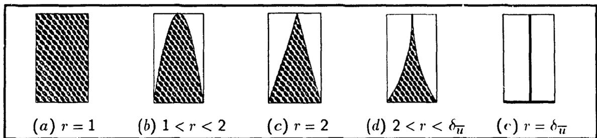
**Figure 4.10** The five possible types of peak shapes described by the shape factor  $r$  for given  $\bar{k}_{\sigma max}$  and  $\delta_{\bar{u}}$ . In (a)  $\bar{k}_{\sigma avg} = \bar{k}_{\sigma max}$ . In (b), (c) and (d) are shown the three most common types of curvature peaks. In (e)  $\Sigma \bar{k}_{\sigma} \approx \bar{k}_{\sigma max}$ .
