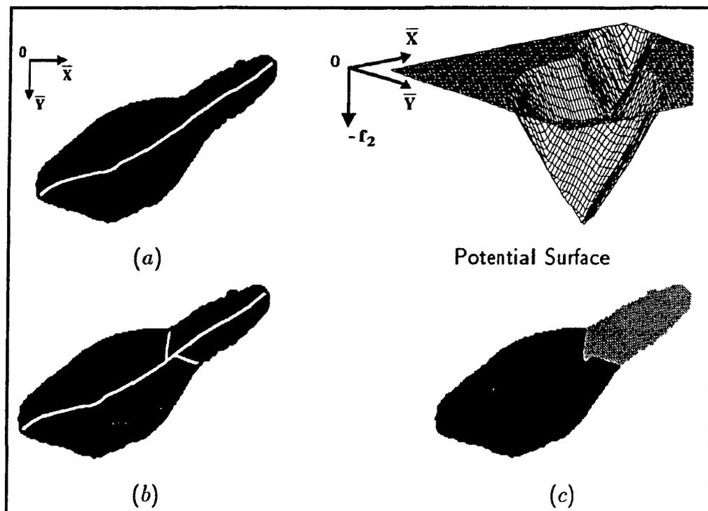
**Figure 5.13** Example of the use of concavities for shape segmentation in the case of a shape of a cell. The usual skeleton generated for the two most significant convexities is shown in (a). Two branches are added in (b) by growing snake segments from significant concavities. In (c) is shown the segmentation of the cell shape into its two main parts, that is, the cell body (in black) and its pseudopod (in grey).
