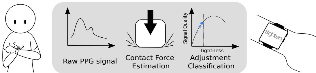
**Fig. 7.2** Visual representation of TightHR used in a tightness recommendation system. 1) A user is putting a wearable on. 2) Signals from the optical heart rate sensors are acquired. 3) Contact force is estimated from the properties of the signal's waveform. 4) Tightness of the band is classified. 5) Feedback is presented to the user who adjusts the tightness as needed.
