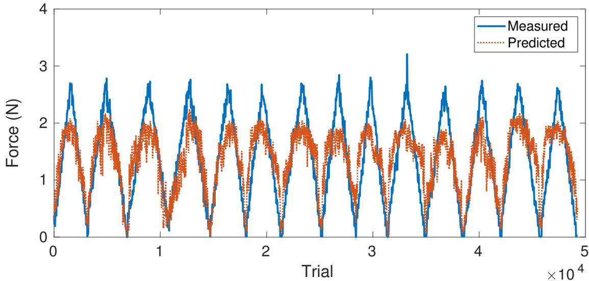
**Fig. 5.3** Visual comparison of measured and predicted forces across the measurement sessions. Sensor saturation visibly begins at approximately 1.5 N.
