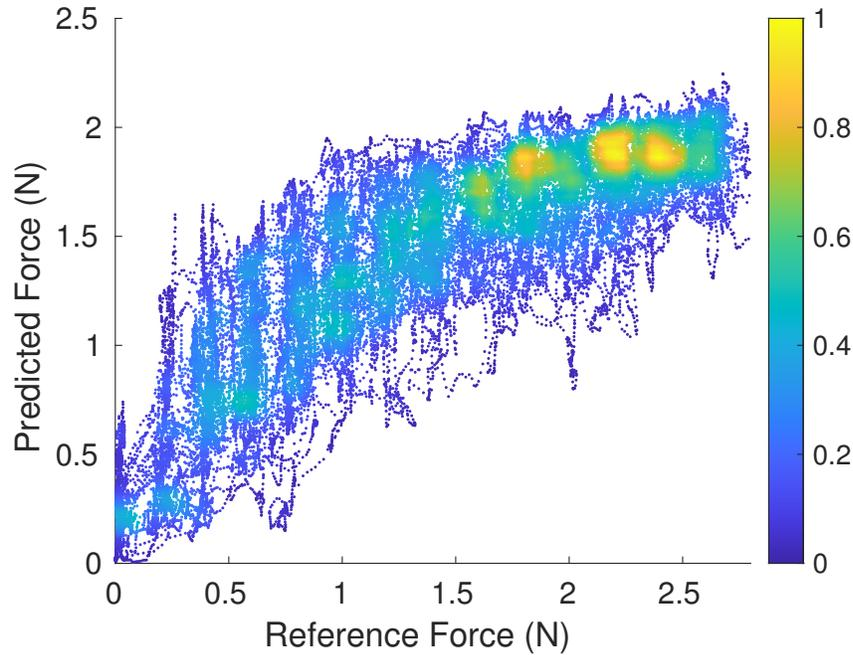
**Fig. 5.4** Contact force estimation model characterization with relative density colormap
