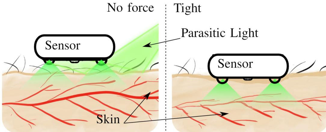
**Fig. 5.1** Increased contact force compresses the tissues, blood vessels and correspondingly modifies the reflected light's properties.
