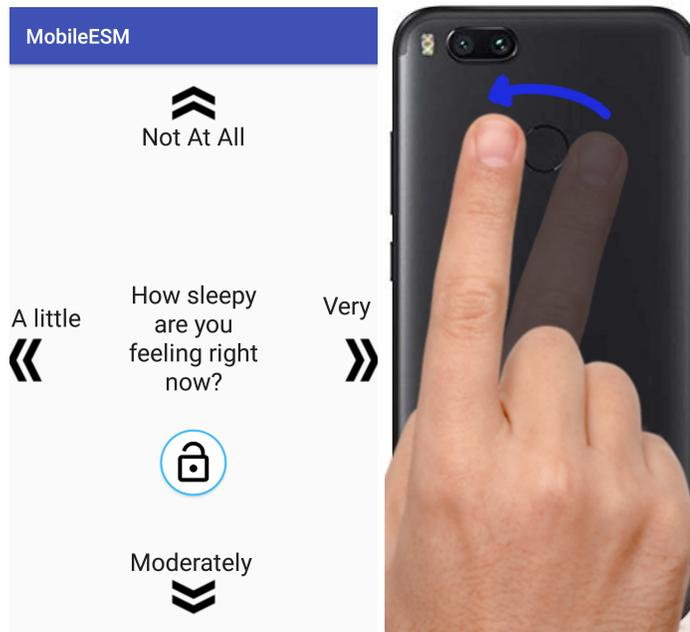
**Fig. 6.1** Screenshot of the fingerprint sensor gesture interface and example gesture required to enter "Very". The inversion of the swiping gesture is due to it being applied to the back of the device
