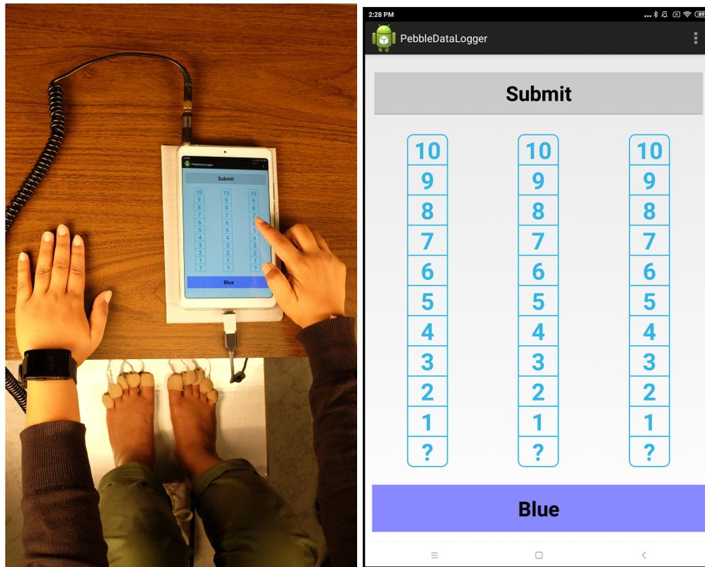
**Fig. 4.3:** Experiment setup and tablet UI for entering responses. In the experiment, the feet are obscured by the table, included here for illustration purposes.
