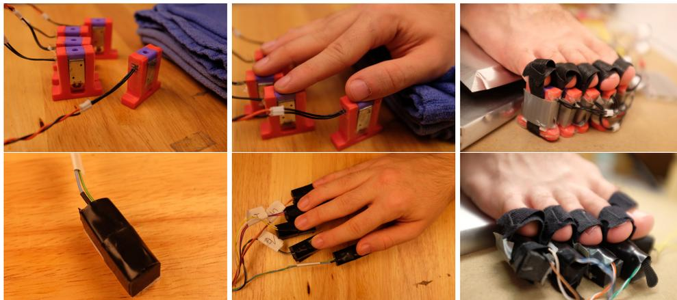
**Fig. 3.2:** Hardware setup for rendering poking (top panel) and vibration stimuli (bottom panel).
