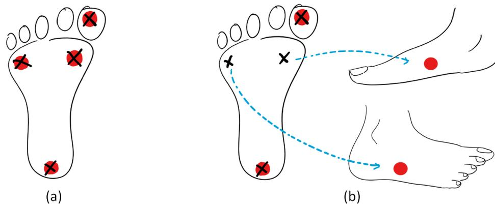
**Fig. 5.2:** Placement of actuators and force sensors. The actuators are marked by red dots and the force sensors are marked by crosses (X). Sub-figure (a) shows the placement used by Anlauff *et al.* [2] whereas (b) shows our proposed placement incorporating the dorsal side.
