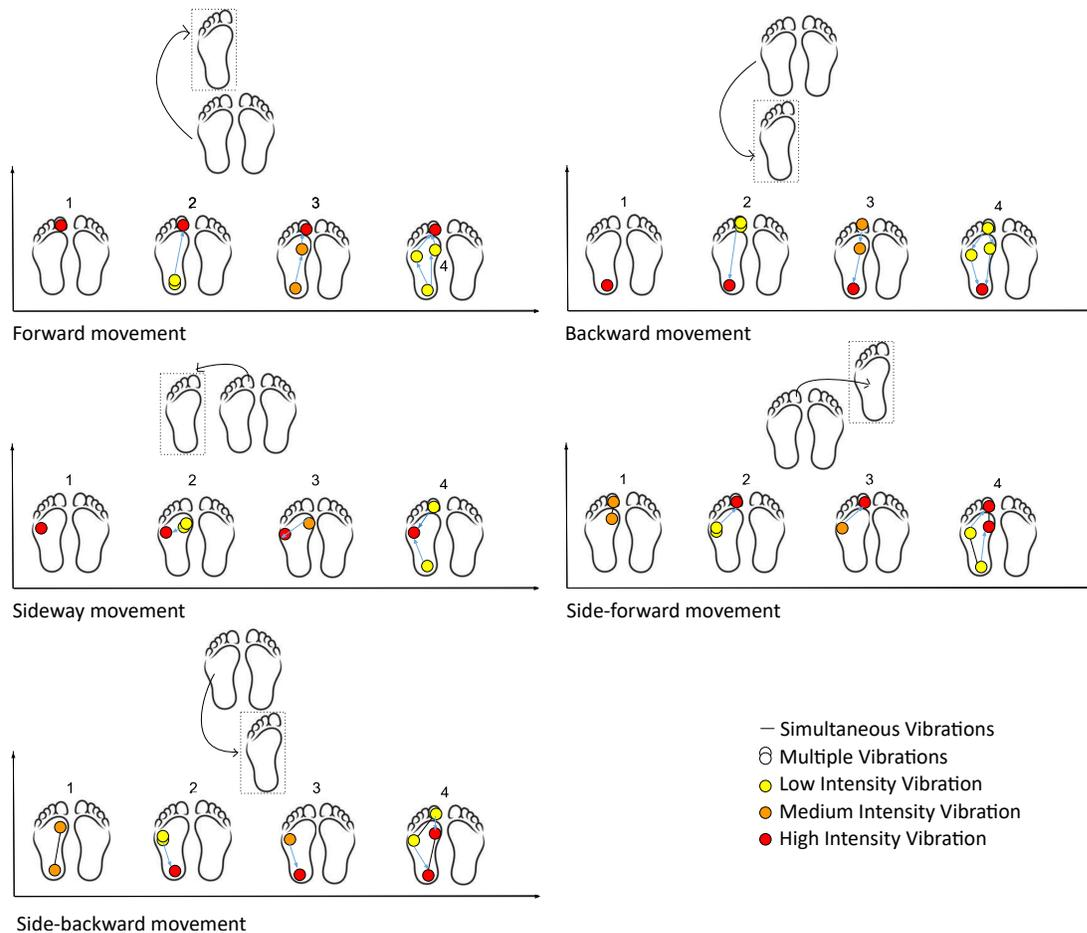
**Fig. 5.4:** Sample haptic patterns to convey basic steps of Salsa. Pattern 1 has vibrations directly mapped to the direction of foot movement. Patterns 2 and 3 have vibrations that lead to a particular direction from the opposite side and hint movement along a line. Pattern 4 creates a gradient vibration using almost all the actuators for conveying a direction; this might have a sweeping effect.
