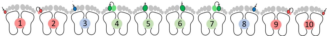
**Fig. 4.2:** Final design of HapToes for both feet. For numbers 1, 3, 5, 6, 8 and 10, a long vibration of 1200 ms is rendered on the targeted toe (darker color). For the remaining numbers 2, 4, 7 and 9, a short vibration of 400 ms is rendered on the closest edge toe, followed by a longer vibration of 800 ms on the targeted toes (darker color).
