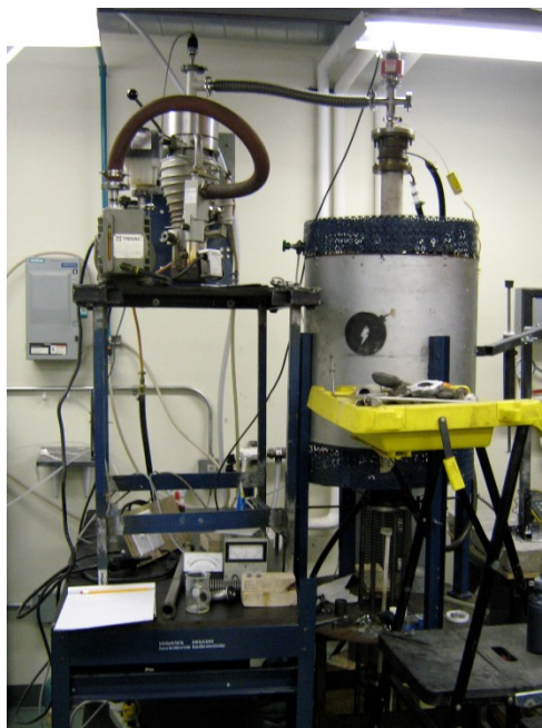
Figure 4-2 : Vacuum furnace utilized to sinter slip cast Inconel 718 and CGDS deposits
