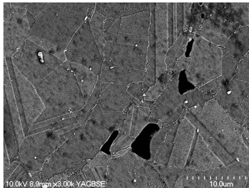
a) CGDS sample sintered at 1200 °C for 10 min; the grains are recrystallized and present MC carbides.
