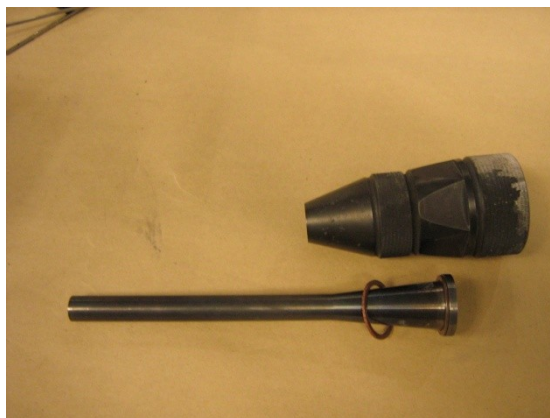
Figure 4-3 : CGDS deLaval nozzle and fixture used to cold spray Inconel 718
