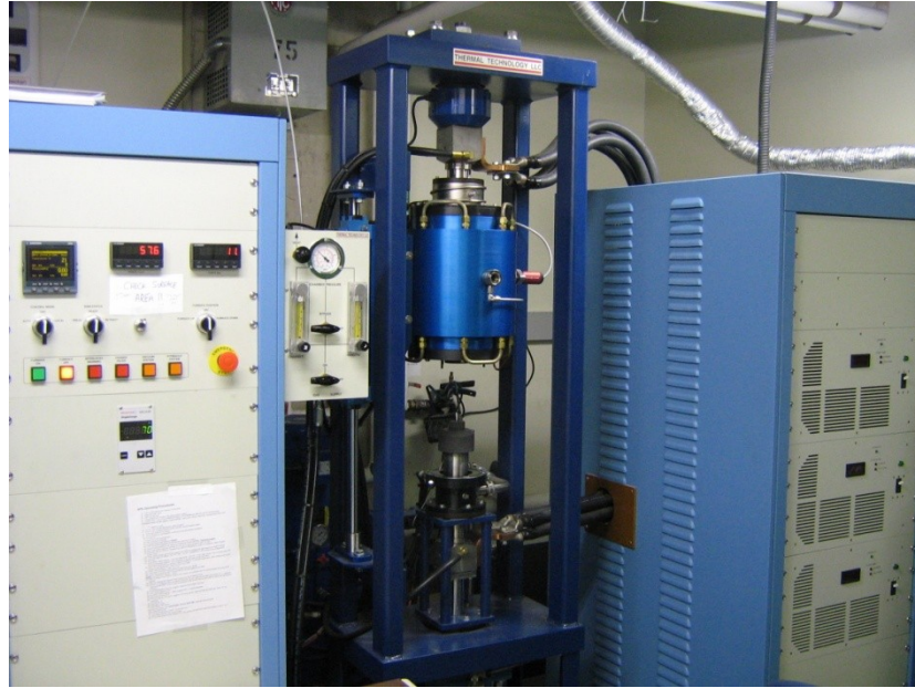
Figure 4-4 : Thermal Technology LLC 10-3 SPS press used to sinter Inconel 718 powder in the SPS and FPSPS experiments
