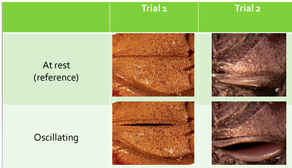
Figure 3.4 Images obtained of vocal folds at rest and oscillating during 2 successful trials of Digital Image Correlation.
