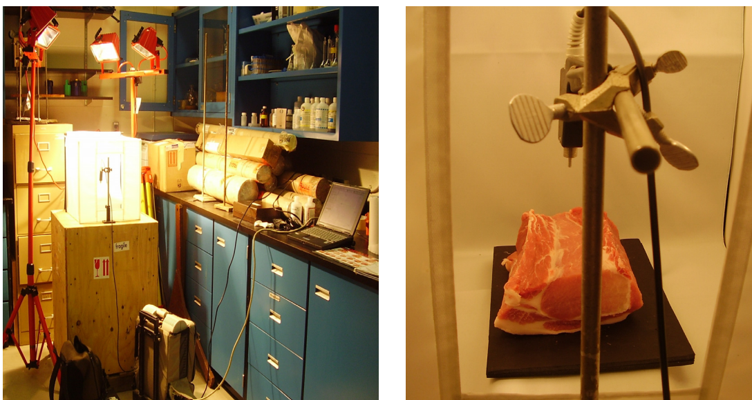
Figure 5.2 Spectroradiometer and experimental setup.
