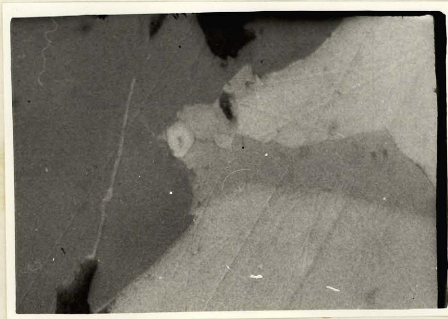
Figure 33 - Tetrahedrite veinlets (medium gray) in galena (light gray) and sphalerite (dark gray) x550.
