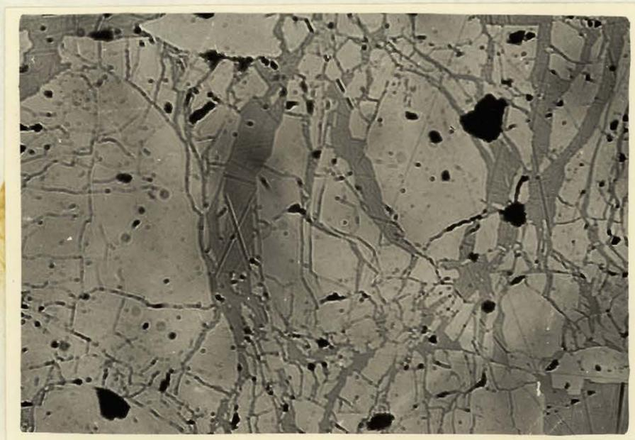
Figure 16 - Galena (medium gray) veining pyrite (lighter gray) x100.
