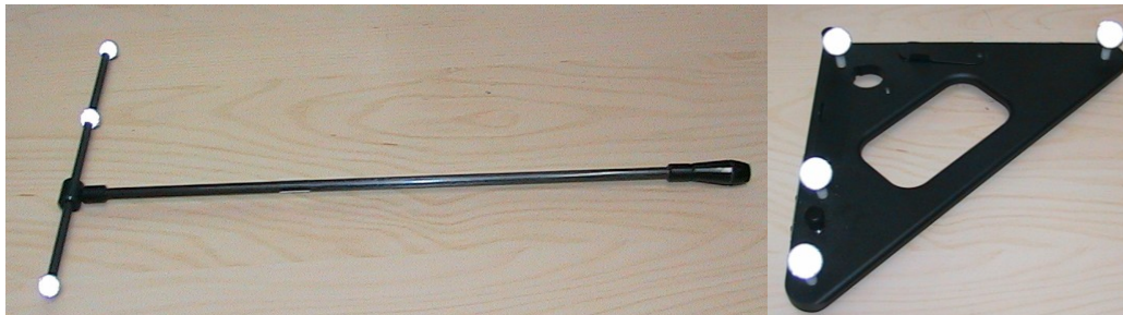
Fig. 3.5: a) 14 mm markers dynamic calibration wand b) 30 mm markers L-Frame for origin calibration
