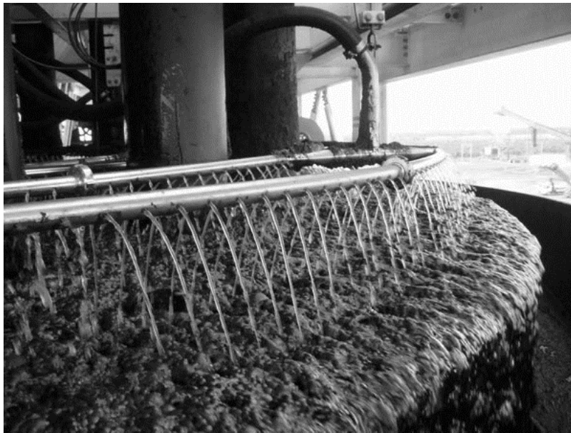
Figure 3: Wash water system in Jameson Cell for coal flotation[8]
