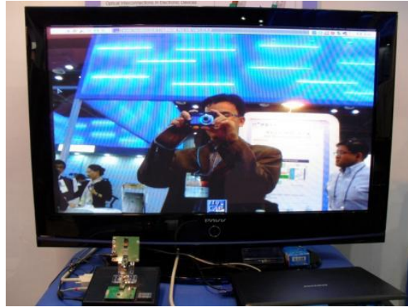
Fig. 2.12. The mobile phone camera records HD digital image then the image data is transmitted to the LCD using the LRSPP interconnect [26].
