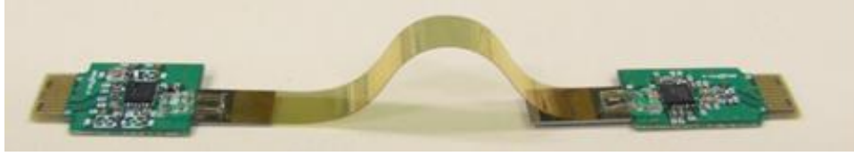
Fig. 2.11. The flexible plasmonic waveguide connecting transmitter and receiver ICs [26].
