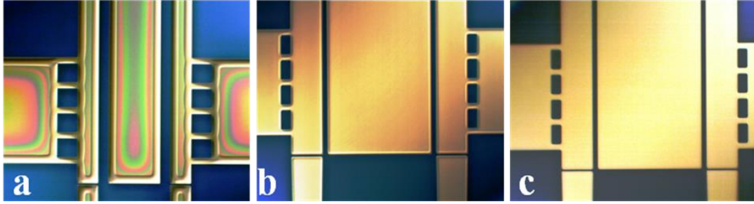
Fig. 4.10. The effect of top cladding thermal processing on the first metal layer of the device (50× magnification) where Cytop is hard-baked at 90 °C: (a) without a thermal ramp, (b) with a 10 °C/hr thermal ramp, and (c) with a 5 °C/hr thermal ramp.
