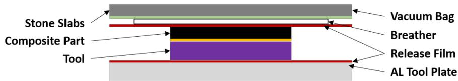
Figure 3.19: General assembly for the WLVB process.
