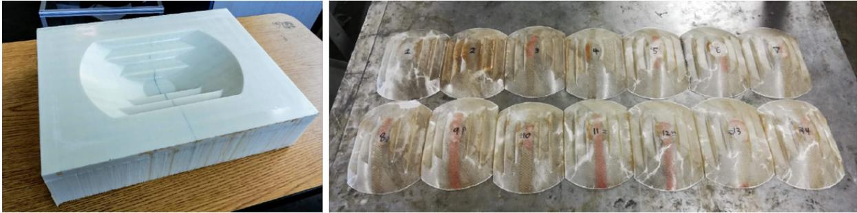
Figure 2.23: Tool durability testing through repetitive use of tool to produce parts. Adapted from [17].
