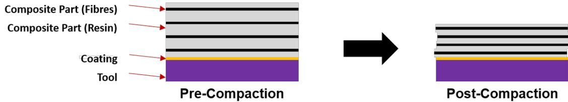
Figure 4.22: “Free-floating” edge effect during ply compaction leading to misaligned plies.
