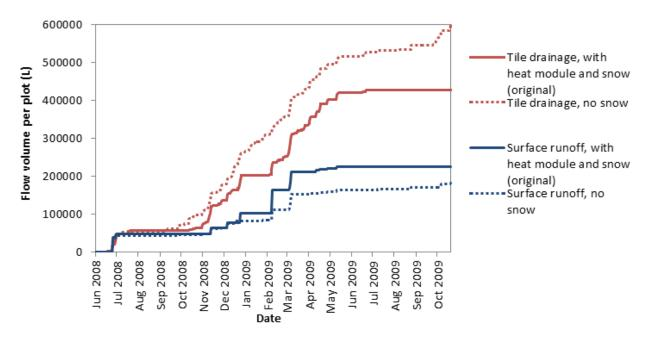
Figure 4.7 Water flow simulation in plot 9 as affected by heat transport and snow accumulation functions.
