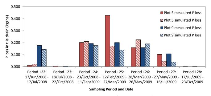
Figure 4.3 P loss in tile drainage, simulated from June 17<sup>th</sup>, 2008 to Feb 11<sup>th</sup>, 2009. Model calibration consisted of periods 122 to 124, model validation consisted of periods 125 to 128.
