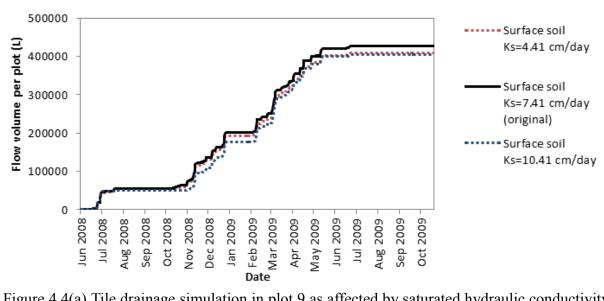
Figure 4.4(a) Tile drainage simulation in plot 9 as affected by saturated hydraulic conductivity  $(K_s)$  in surface soil layer.
