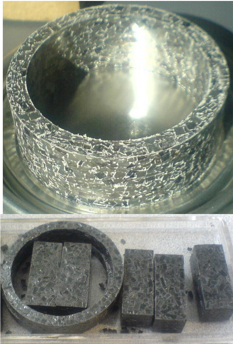
Figure 38: Example of SL-SMC parts, cold pressed, using the optimum conditions developed to date (0.75 wt% Lub), and exhibiting a good surface finish.
