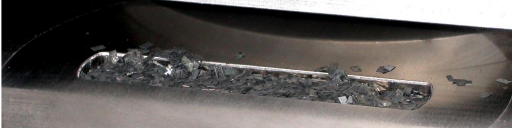
Figure 69: Top of the die cavity when the feed shoe retracts, showing lamellae expelled from the die.
