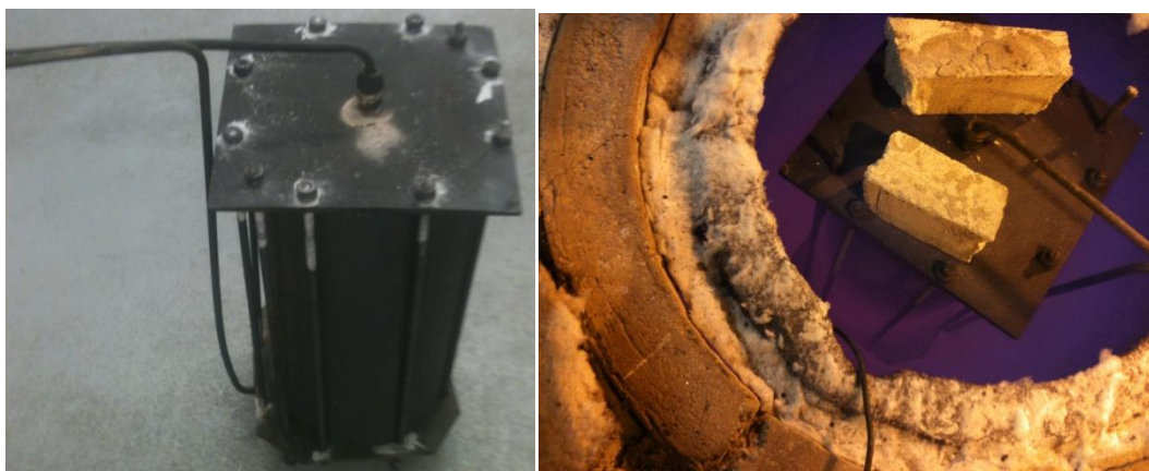
Figure 29: Left: Stainless steel retort developed to carry out thermal treatments under a reducing atmosphere on rolls of ribbon at the MMPC, using a tilting electric element heated casting furnace (Pyradia model B7D363625SV). Right: The retort is in the furnace at high temperature and the top cover of the furnace was removed quickly to take the picture.
