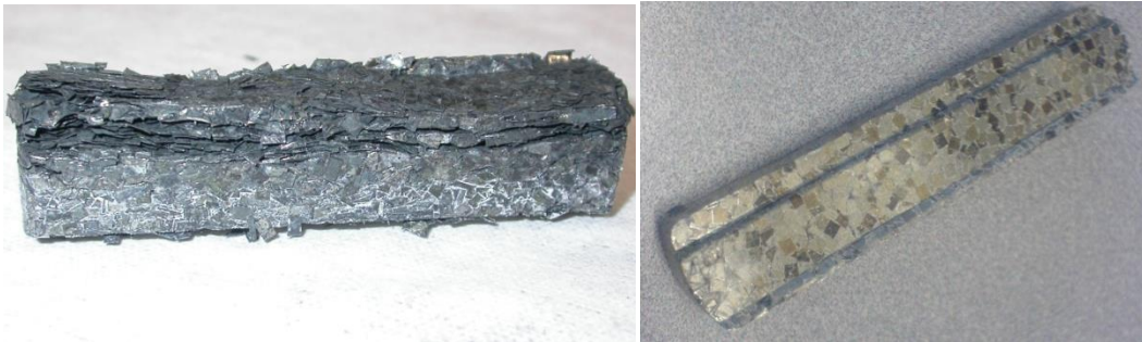
Figure 66: De-lamination observed on parts compacted using strain hardened lamellae particles (Fe-Co) and conventional lubricant (left) and (right) the good surface finish obtained with a polymeric binder and soft particles.
