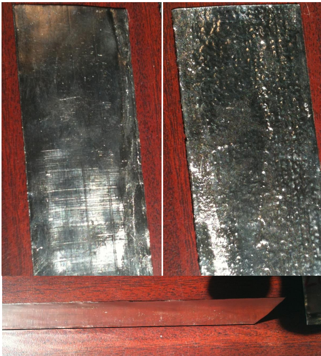
Figure 56: Tin casting results, (top left; wheel side, top right; free surface side, bottom, side view to appreciate the thickness and planarity). 4 mm contact length, 500 \mu\text{m} gate opening, 45 K superheat, 2.5 m/s wheel speed.
