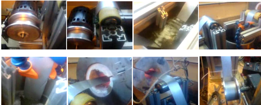
Figure 27: Cleaning line developed to prepare the surface of the ribbons (remove traces of oil) prior to the annealing/grain coarsening thermal treatment and the coating operation. From left to right, up line: un-coiler with its brake to keep a certain tension in the ribbon during the cleaning cycle, ultrasonic bath intake roll, bath immersed roll, exit of the bath and the set up for the rinsing bath. Down line, the two rinsing nozzle at the exit of the rinsing bath, the intake of the drying furnace, the exit with its air knife, and the re-coiler.
