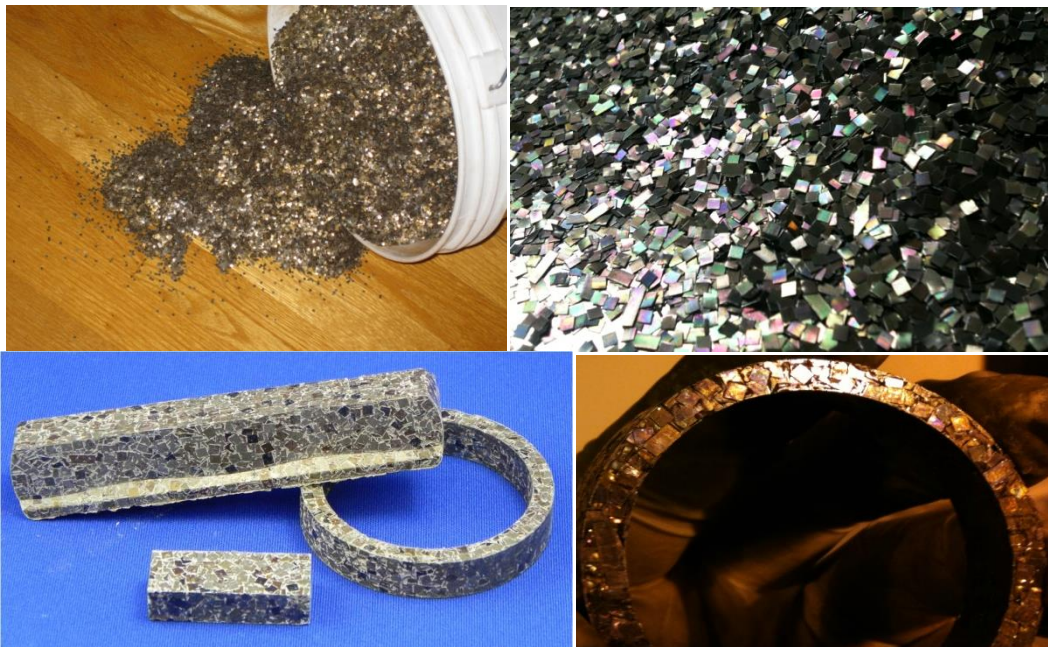
Figure 37: Powder produced with the new SL-SMC process and an example of a part pressed for characterization (small rectangle and the ring) or motor teeth pre-form ready for forging.
