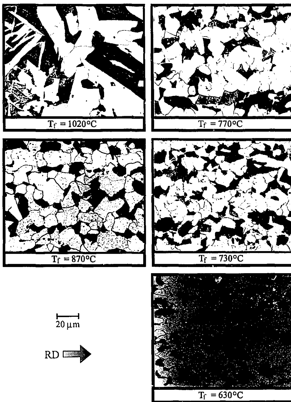
Figure VI.3 Optical micrographs of the plain carbon steel, austenitized at 1250°C and hot rolled to 75% reduction at several finish rolling temperatures. 2% nital etch.
