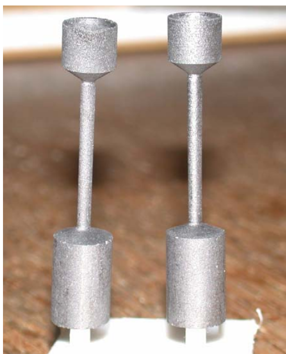
Figure B-8. Used (left) and new (right) graphite cups.
