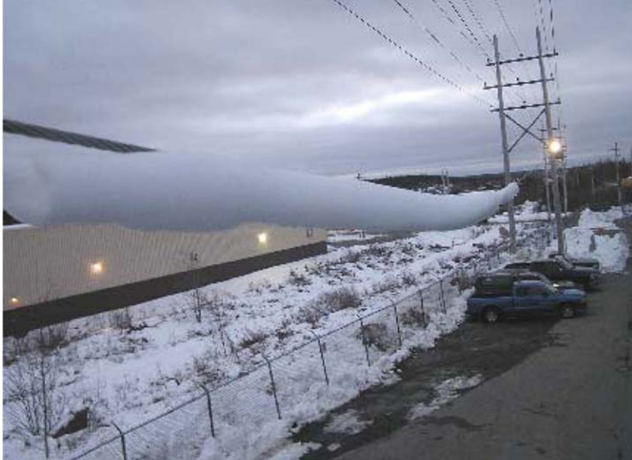
Fig.12 Wet snow sleeve still holding to a wire, November 17 th , 2004 (from the report issued on January 18 th 2005 by the Nova Scotia Utility and Review Board on the wet snow storm of November 13 th and 14 th , 2004)
