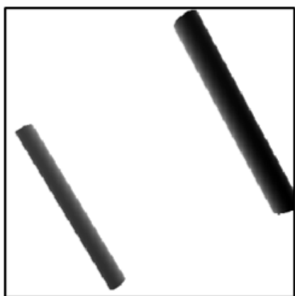
Figure 4.8: Input depth image from 3 meters above logs
