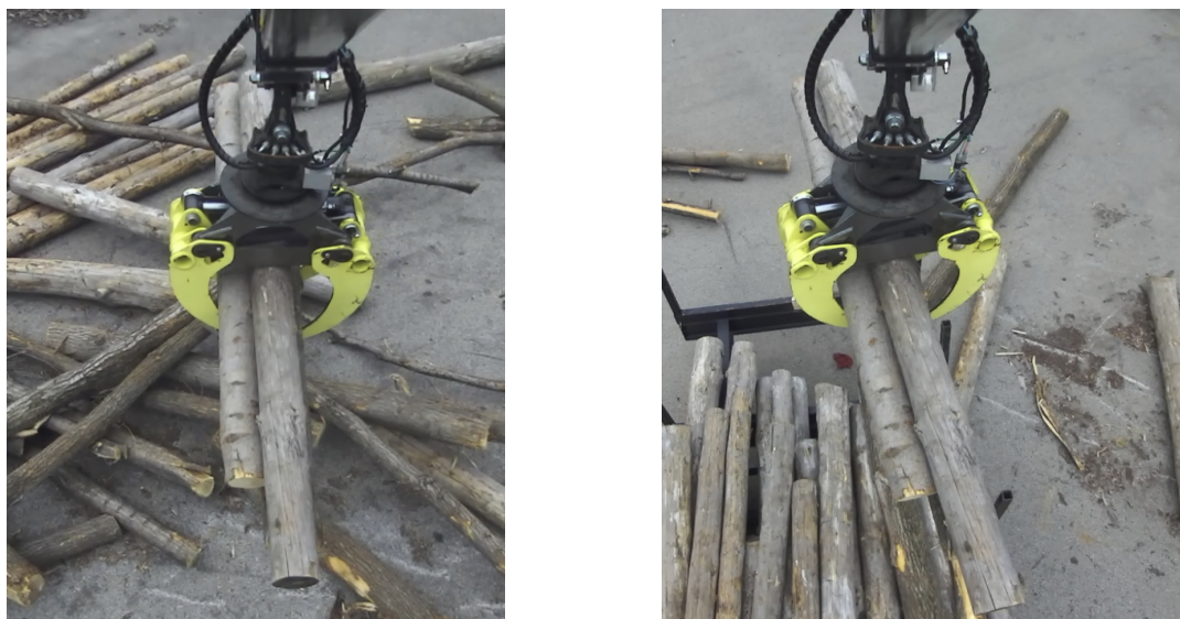
Figure 5.18: Grapple with three grasped logs, one of which is hidden
