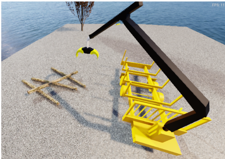
Figure 4.7: Log-loading test-bed Isaac Sim simulation environment
