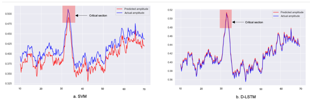
Figure 6.20: Performance comparison of baseline (SVM) and Proposed model (D-LSTM)
