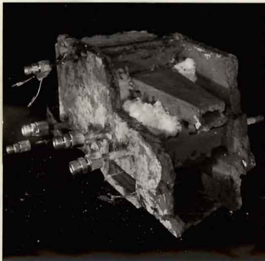
Fig. 44. Main casting broken open, showing ejector
