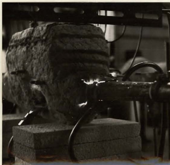
Fig. 40. Inlet section leaking
