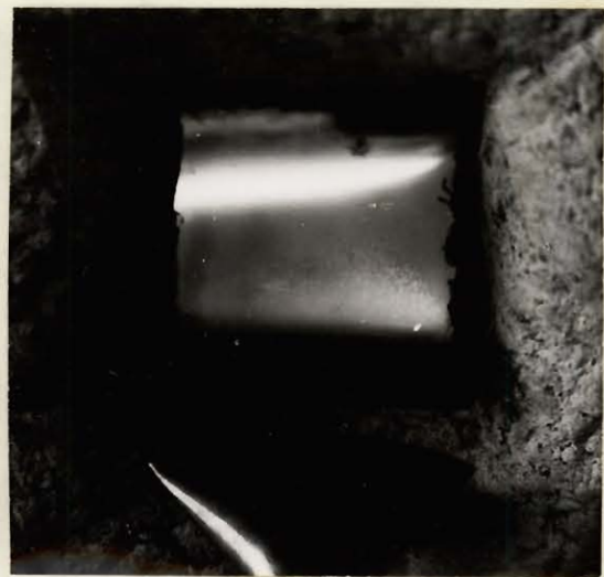
Fig. 35. Secondary combustion at mixing surface - rich mixture
