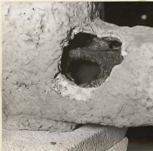
Fig. 34. Hole in exhaust section; Bacite removed.
