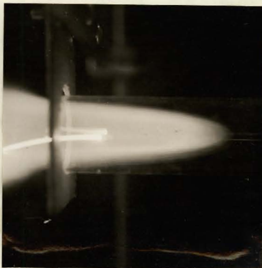
Fig. 14. Flame stabilized inside large tube
