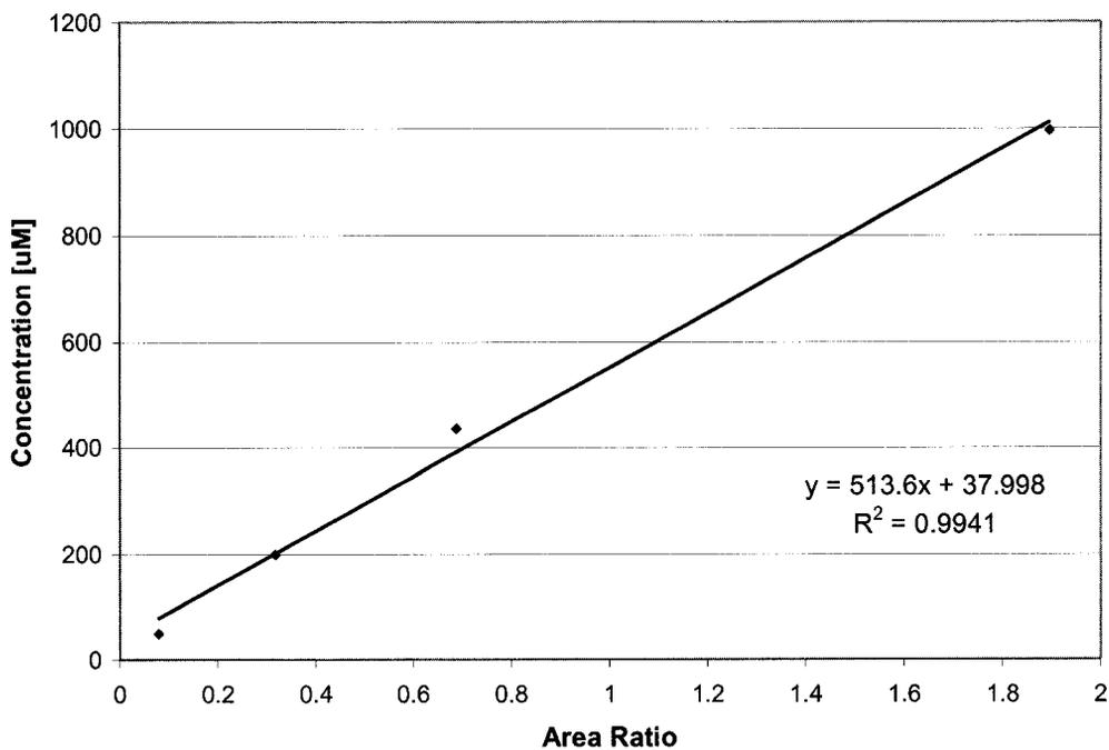
Figure 5.2 DEHA calibration curve
