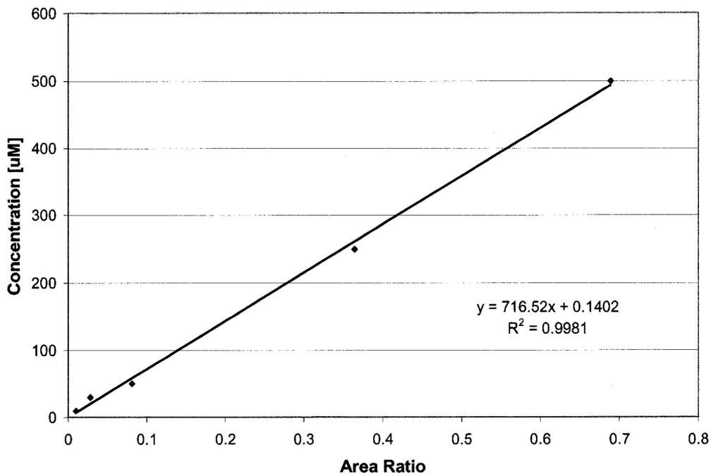
Figure 5.4 2-Ethylhexanol Calibration Curve for 100 to 500 uM
