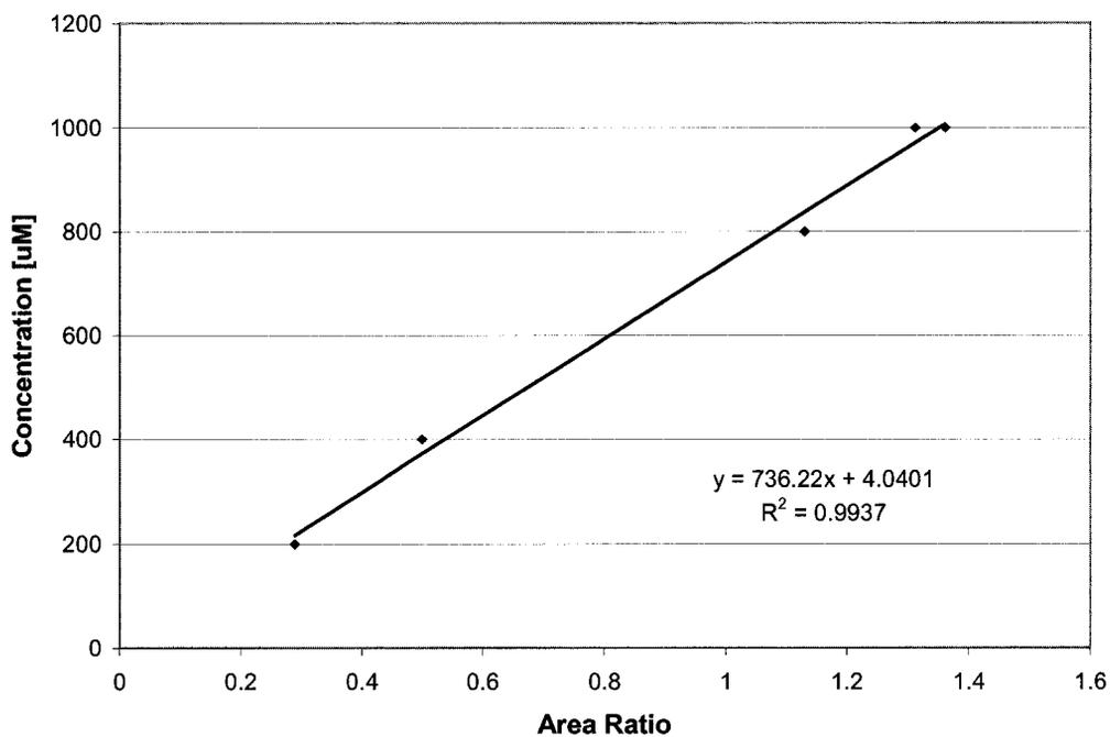
Figure 5.5 2-Ethylhexanoic Acid Calibration Curve
