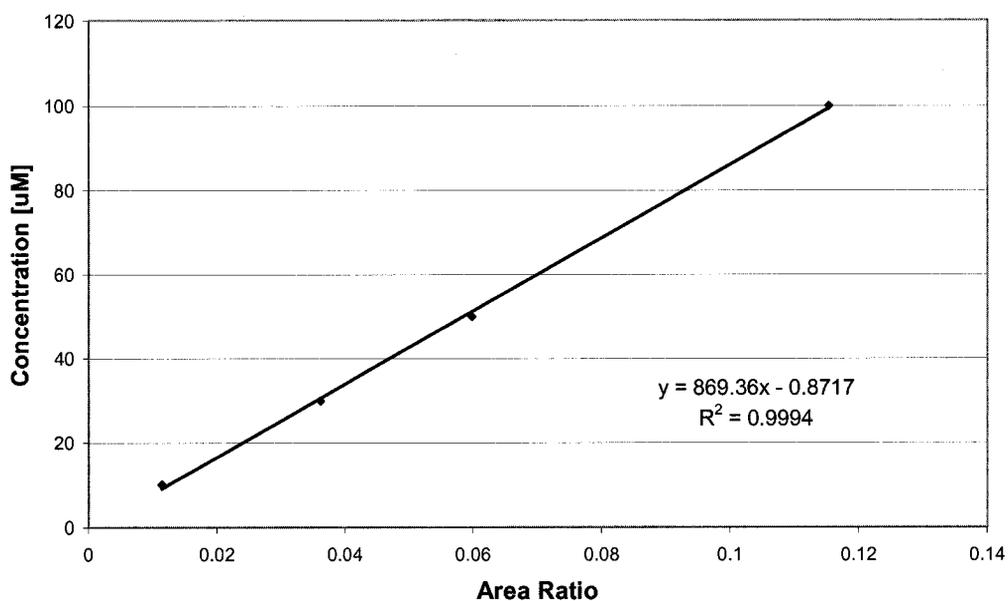
Figure 5.3 2-Ethylhexanol Calibration curve for 10 to 100 uM
