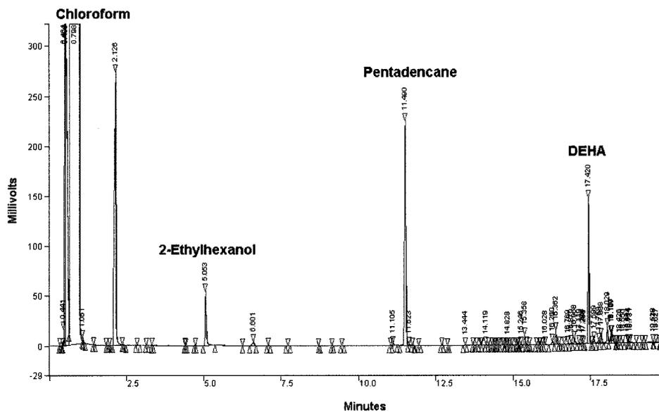
Figure 5.1 Typical Gas Chromatograph, Varian CP 3800, FID detector, column CP SIL 8CB
