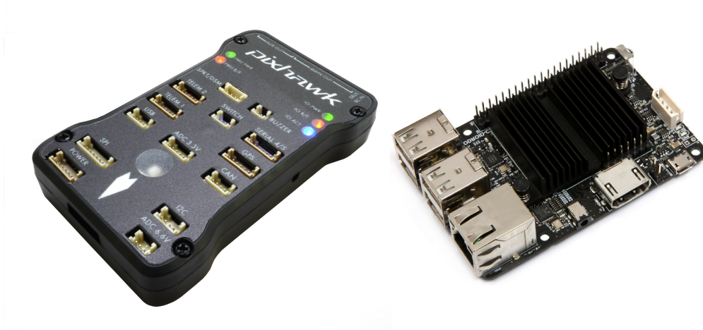
Figure 3-4: Pixhawk microcontroller and Odroid X4U Linux computer
