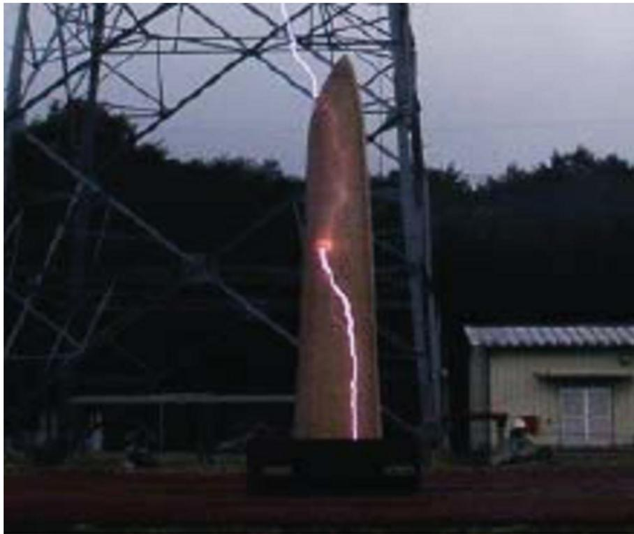
**Figure 9 - Lightning discharge on wind turbine blade**
